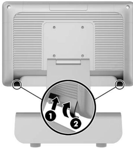
2. Disconnect all cables from the rear I/O connectors, including the power cord.
