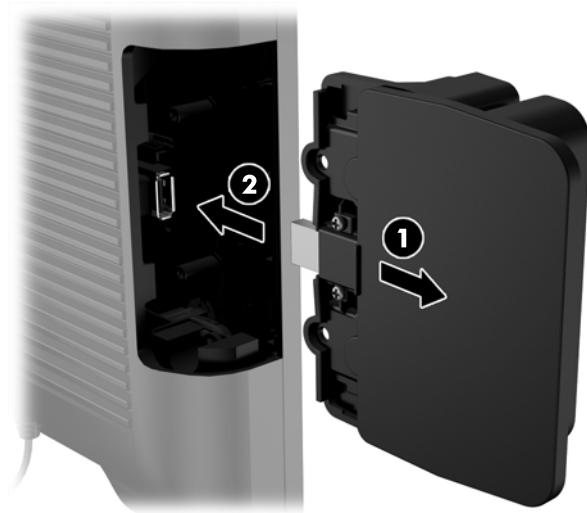
7. Install the two screws that were previously removed (1) and slide the cover plate on the module forward to cover the screws (2).
