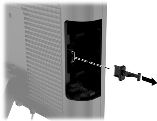
5. Remove the two screws next to the USB port. The screws are needed to install the USB module.
