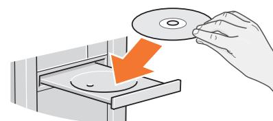
**EN** Install the product software from the DVD that came with your printer onto your computer. Be sure to follow the software installation instructions. For USB connections: Connecting your product before installing the software can lead to product errors.
