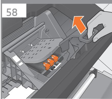
EN Lift the handle up to open the printhead cover. The front panel prompts you for the next step: removing the printheads. Do not press OK until you have removed all the orange setup printheads.
