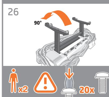
**EN** Rotate the product 90 degrees. **IMPORTANT:** make sure that the roll feeds are facing downwards.
