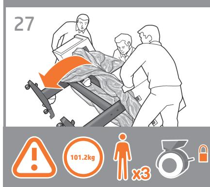
**EN** Hold the product by the foam end pieces and by the center rear, and rotate it until it stands on its feet, with all four wheels in contact with the floor. The product weighs 101.2 kg (223 lb).
