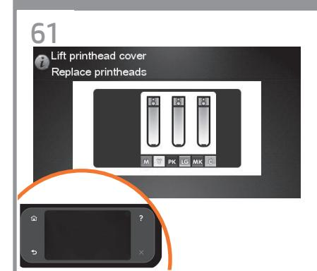
Press the OK key on the front panel when you have removed all of the setup printheads. The front panel then prompts you to install the new printheads.
