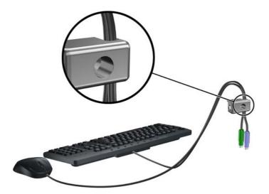
6. Screw the lock to the chassis using the screw provided.
