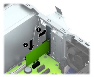
NOTE: When installing an expansion card, press firmly on the card so that the whole connector seats properly in the expansion card slot.
