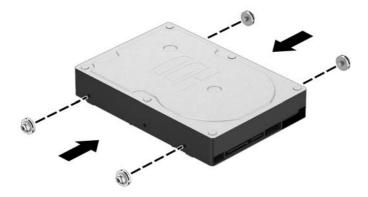
• If installing a hard drive in the lower (primary) drive bay, remove the silver and blue mounting screws from the old drive and install them in the new drive.
