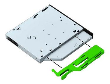
9. Slide the optical drive all the way into the drive bay (1) until the green latch locks onto the bottom of the drive bay (2).
