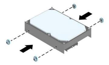
8. Slide the drive into the drive bay, making sure to align the mounting screws with the guide slots, until the drive snaps into place.
