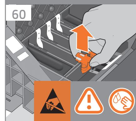
Remove and discard all orange setup printheads. You may need to use force to extract each printhead. The setup printheads contain ink, which could leak out. Avoid touching pins, leads or circuits.
