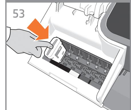
**EN** Insert the ink cartridges one by one. Each cartridge is marked with its own color, and should be inserted only into the slot of the same color. Avoid touching pins, leads or circuits.
