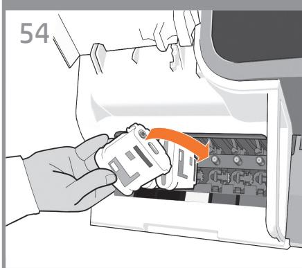
**EN** The cartridges must be inserted the right way around: the ink outlet in the cartridge should meet the ink inlet in the slot. Push the cartridge into the slot until it clicks into place. The product beeps whenever a cartridge is successfully inserted.
