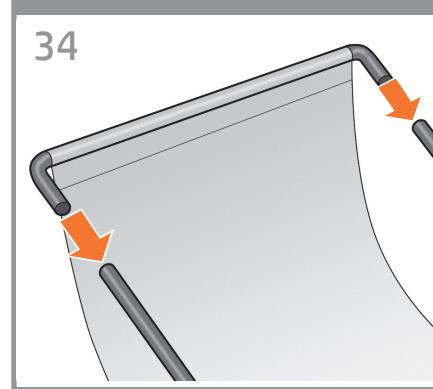
**EN** Attach the basket's front tube to the two short tubes on each foot.
