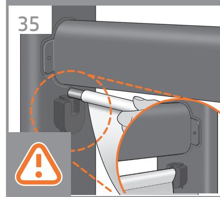
**EN** Rest the basket's rear tube on the supports that you have just fitted to each leg of the stand.
