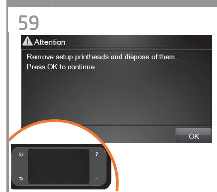
The setup prinheads exist only to prevent the escape of ink during ink cartridge installation. The front panel now prompts you to remove the setup prinheads and press the OK key when you have finished.
