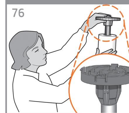
If the blue removable stop is on the spindle, remove it. Put the roll onto the spindle, making sure to put it on the right way round: the leading edge of the paper should go into the product from the top of the roll. Add the removable stop to the spindle to keep the roll in place.
