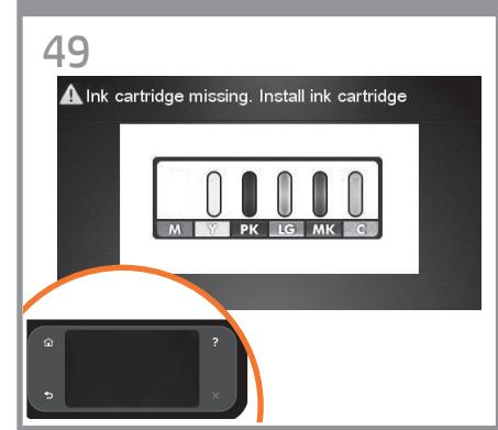
The product checks for the presence of ink cartridges. On finding none, it prompts you to install the ink cartridges.
