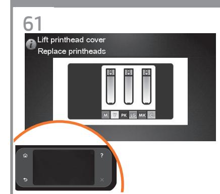
Press the OK key on the front panel when you have removed all of the setup printheads. The front panel then prompts you to install the new printheads.
