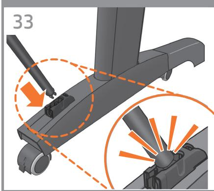
**EN** Fit the two short tubes to the product's feet, one on the front of each foot. Each tube should click into place.
