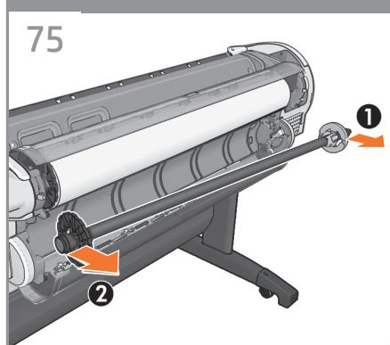
**Remove the spindle by lifting out first the right-hand end, then the left.**
