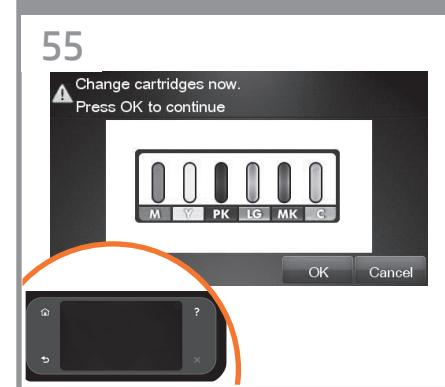
**EN** When you have inserted all of the ink cartridges correctly, the product must prepare the ink system for its first use. It will do this immediately if you press the OK key, or after a 60-second pause if you do not press the OK key. When the ink system is ready, the front panel will prompt you to open the window.
