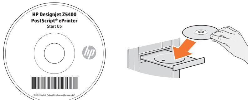
**EN** Install the product software from the DVD that came with your printer onto your computer. Be sure to follow the software installation instructions. For USB connections: Connecting your product before installing the software can lead to product errors.
