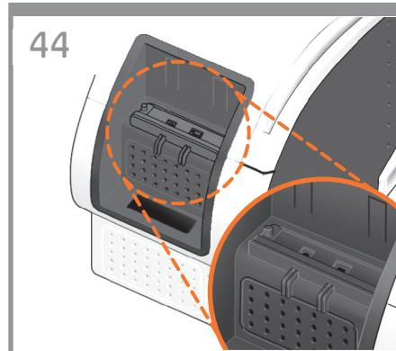
**EN** Connect the network cable or a certified USB 2.0 cable to the appropriate socket on the rear right of the product, and secure the cable with the clip provided, to prevent accidental unplugging.
