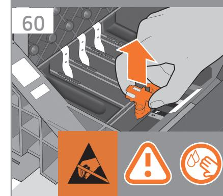
Remove and discard all orange setup printheads. You may need to use force to extract each printhead. The setup printheads contain ink, which could leak out. Avoid touching pins, leads or circuits.
