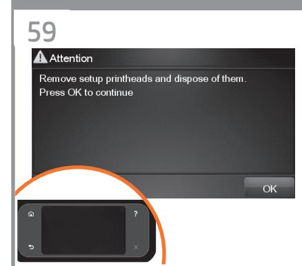
The setup prinheads exist only to prevent the escape of ink during ink cartridge installation. The front panel now prompts you to remove the setup prinheads and press the OK key when you have finished.
