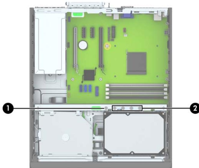
There are a total of five extra silver 6-32 standard screws. One is used for bezel security (1) (see [Front bezel security on page 45](#) for more information). The other four are used as guide screws for a media card reader or a secondary hard drive in the 3.5-inch optional drive bay (2).
