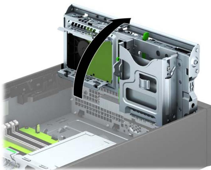
9. Align the guide screws on the drive with the J-slots on the sides of the drive bay. Press the drive up into the drive bay then slide it forward until it locks in place.
