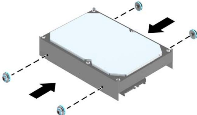
10. Align the guide screws with the slots on the chassis drive cage, press the hard drive down into the bay, then slide it forward until it stops and locks in place.
