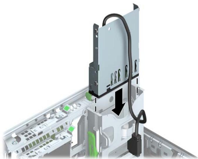
11. If installing a USB 3.0 media card reader, you must use the USB 3.0 to USB 2.0 adapter (1) and connect the adapter cable from the media card reader to the USB 2.0 connector on the system board labeled MEDIA (2).
