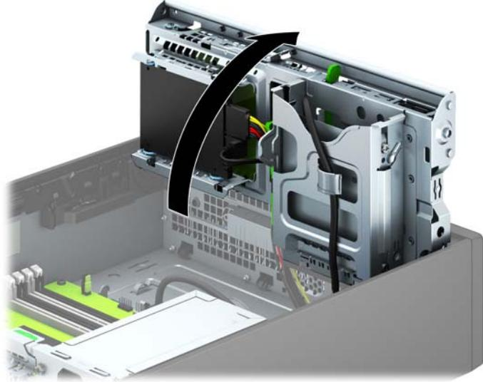
8. Disconnect the drive cables from the rear of the drive, or, if you are removing a media card reader, disconnect the USB cable from the system board as indicated in the following illustration.
