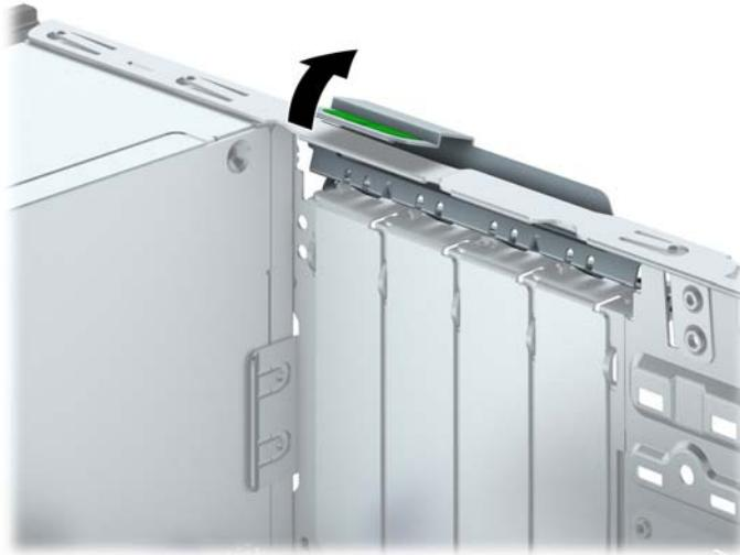
9. Before installing an expansion card, remove the expansion slot cover or the existing expansion card.
