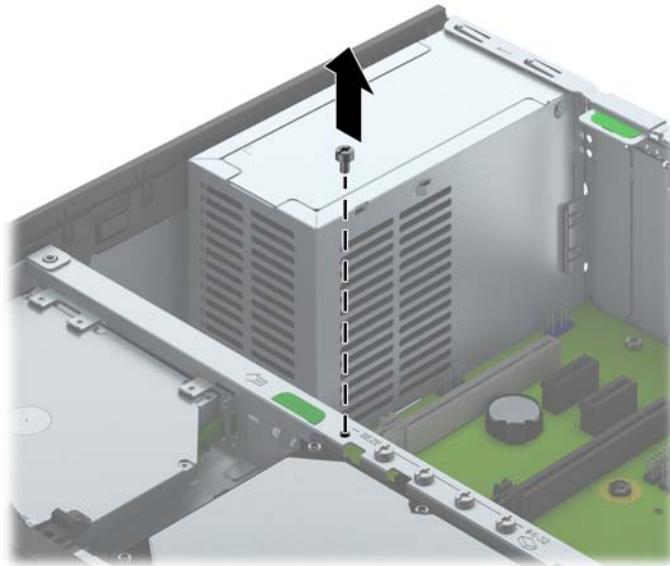
8. Install the security screw through the middle front bezel release tab to secure the front bezel in place.
