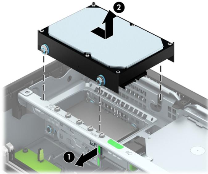
9. To install a 3.5-inch hard drive, you must transfer the silver and blue isolation mounting guide screws from the old hard drive to the new hard drive.
