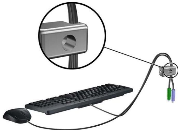
6. Screw the lock to the chassis in the thumbscrew hole using the screw provided.
