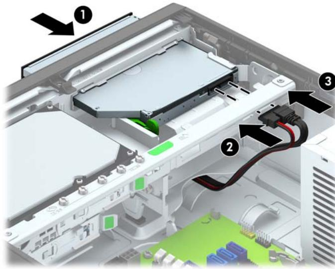
10. Connect the opposite end of the data cable to one of the light blue SATA connectors on the system board.
