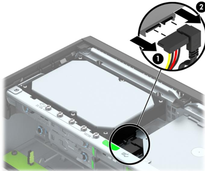
8. Pull the release lever next to the rear of the hard drive outward (1). While pulling the release lever out, slide the drive back until it stops, then lift the drive up and out of the bay (2).
