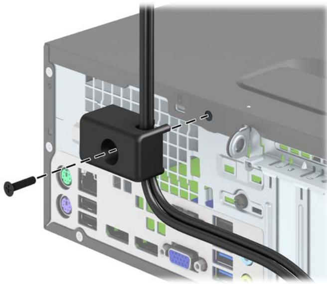
7. Insert the plug end of the security cable into the lock (1) and push the button in (2) to engage the lock. Use the key provided to disengage the lock.
