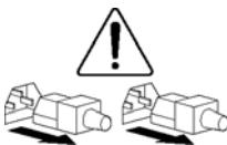
These symbols, on power supplies or systems, indicate that the equipment is supplied by multiple sources of power.
