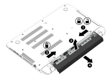
Reverse this procedure to install the battery.
