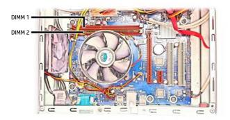
7. Open both latches of the memory module socket (1), and insert the memory module into the socket (2).
