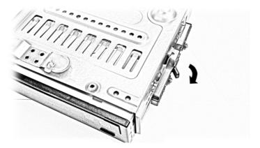
11. Push the optical disc drive out through the front of the cage.
