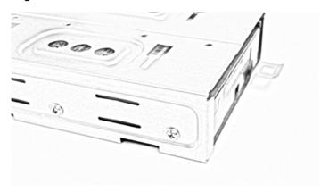
15. Hold the hard drive cage with the connectors next to the power supply and align the openings in the cage bottom with the raised clips on the bottom of the chassis.
