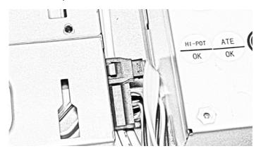
**18.** Connect the opposite end of the data cable to the SATA1 connector on the system board.
