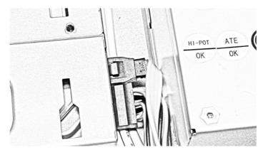
8. Press the tab to disengage the latch securing the hard drive in place.
