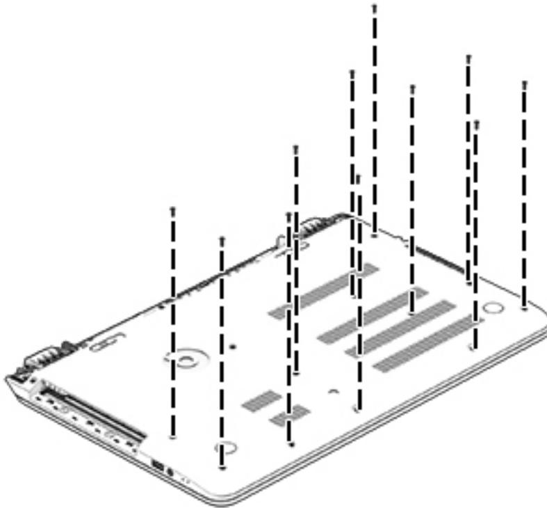
3. Remove eight Phillips screws (1) around the battery area, two broadhead screws (2) in the optical drive bay and one screw (3) near the display hinge.
