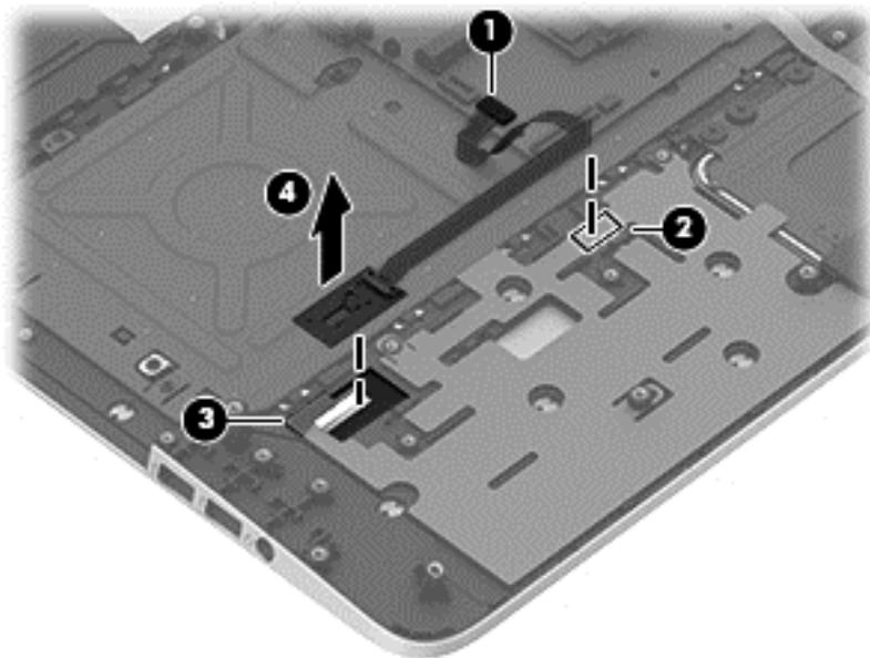
Reverse this procedure to install the fingerprint reader board and cable.
