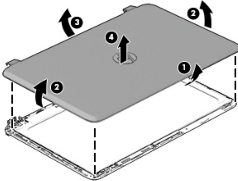
8. If you need to remove the panel, the display cable or the webcam, follow these procedures. To remove the raw panel, remove the six Phillips screws (1) and any adhesive that secures the display panel to the back cover and lift the display panel (2) carefully.
