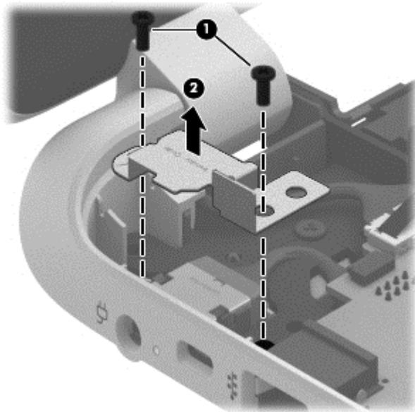
5. Remove the seven Phillips screws (1) on the left and right side base of the display panel and lift the panel up (2).
