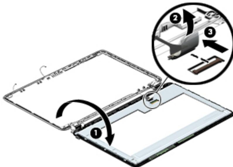
7. Loosen the edges of the back cover (1), (2), and (3) from all four sides of the display bezel and lift the display panel (4).
