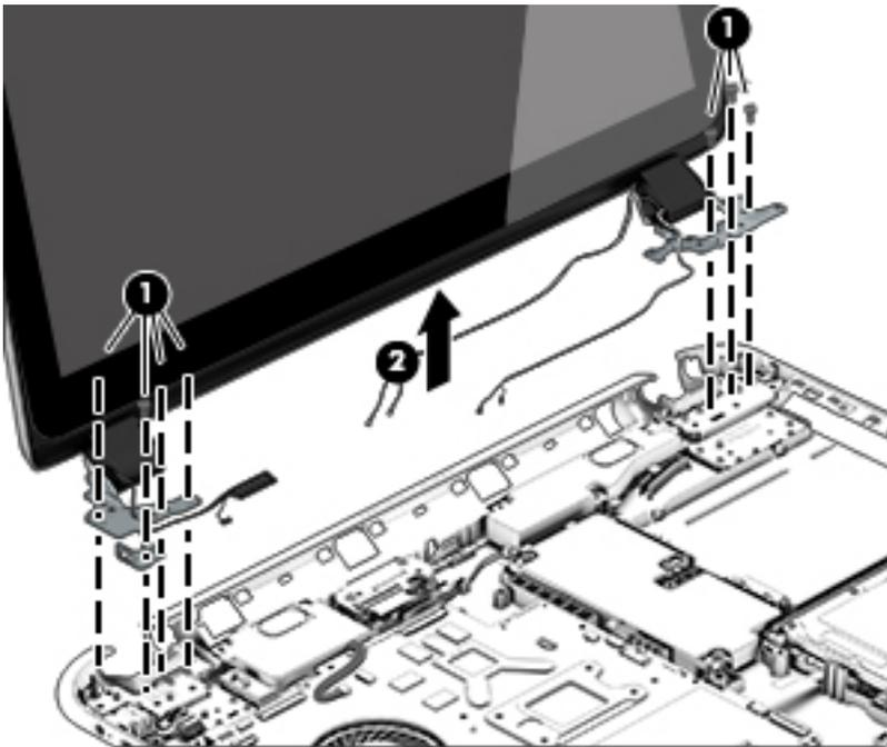
6. Open the panel cover (1), swivel the display panel hinges (2) on both sides and then tilt up the display panel hinge (3) to release it.
