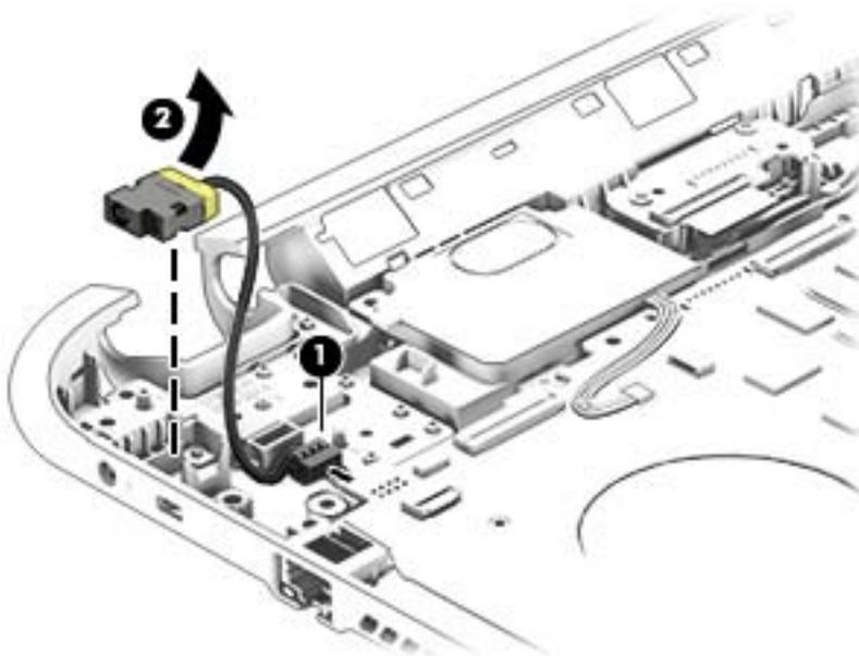
Reverse this procedure to install the power connector cable and bracket.
