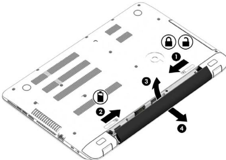
Reverse this procedure to install the battery.
