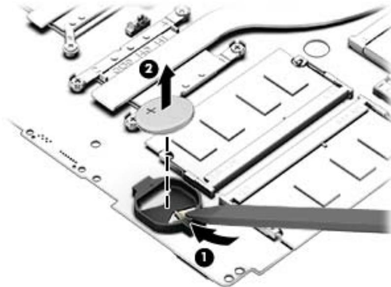
Reverse this procedure to install the RTC battery on computer models. When installing the RTC battery, make sure the “+” sign faces up.
