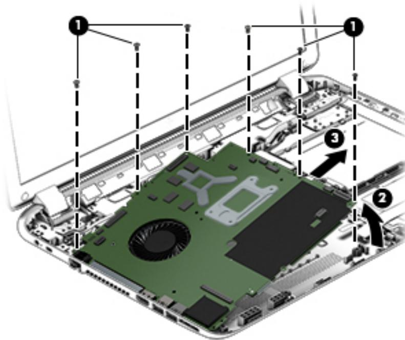
6. Turn the system board over and remove the solid state drive before replacing the system board.
