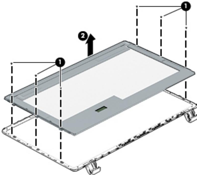
9. Remove the display panel side bracket (select models only) by removing the four Phillips screws (1) and releasing the side bracket (2).
