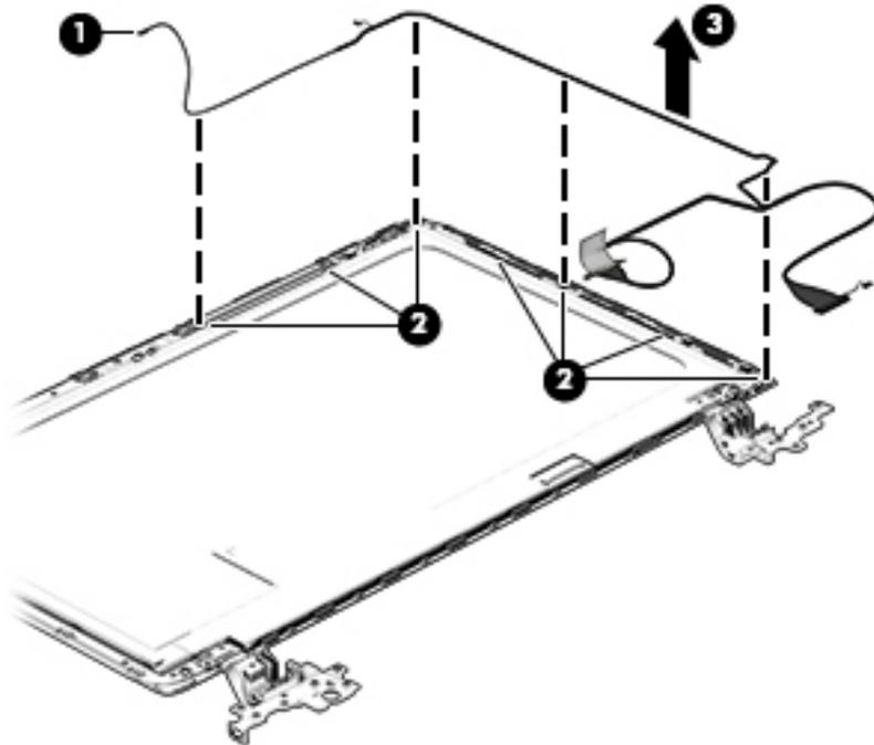
11. On select models, removing the cable also requires disengaging it from the channels in the hinges and disconnecting from the display panel. To disconnect the cable from the display panel, carefully remove the foil tape at the bottom of the display panel and then carefully lift the display cable connector (1) and remove the display connector (2).
