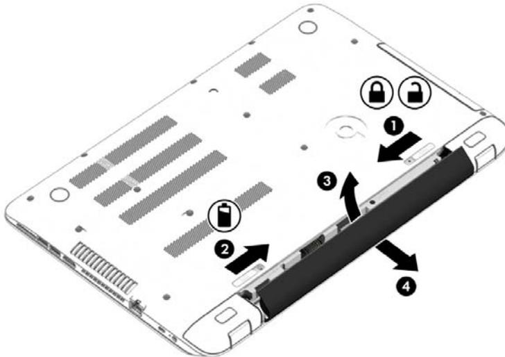
Reverse this procedure to install the battery.
