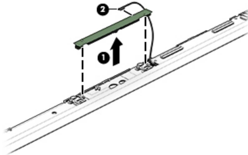
13. If it is necessary to replace the WLAN antenna cable, follow these procedures:
