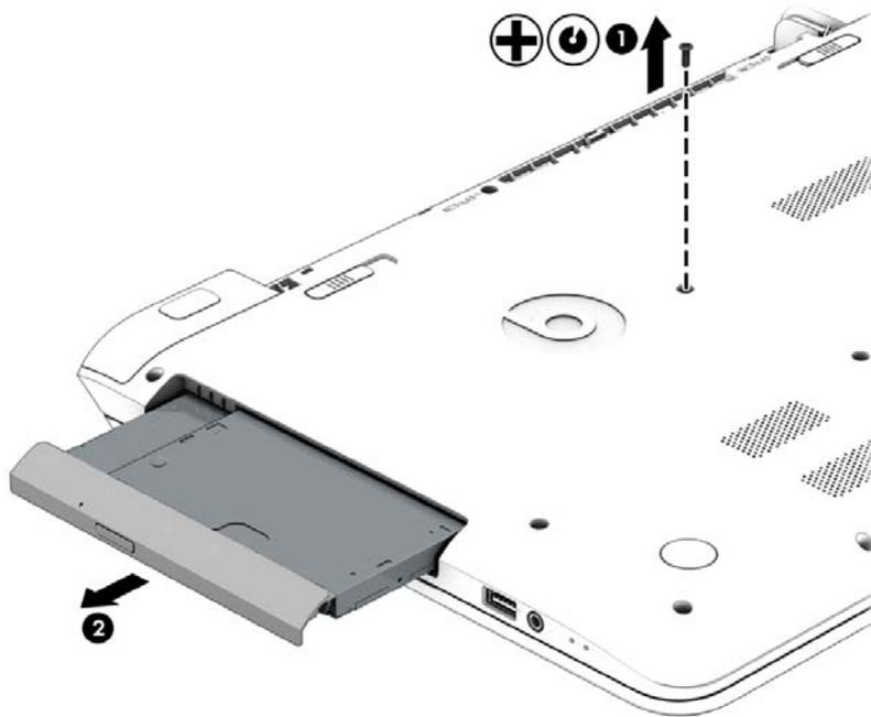
4. If it is necessary to replace the optical drive bracket, position the optical drive with the rear panel toward you.
