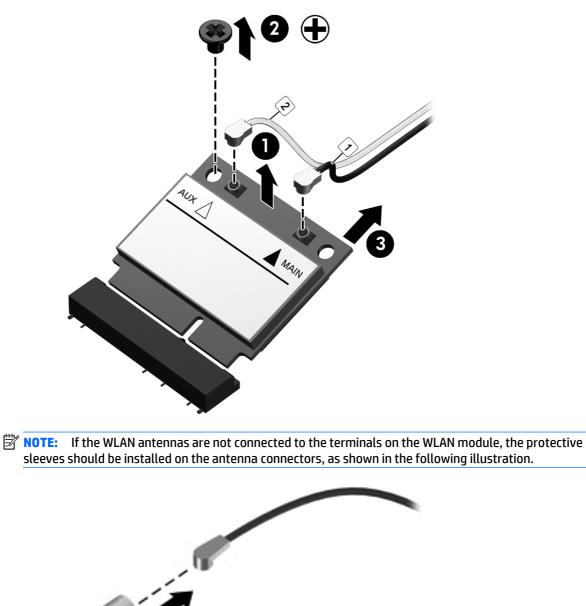
Reverse this procedure to install the WLAN module.
