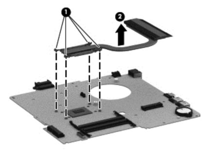
Thoroughly clean the thermal connections (1) on the system board and the heat sink (2) before replacing a heat sink onto a system board.
