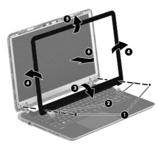
**c.** Remove the four Phillips M2.0×2.5 screws (1) and carefully move the display panel (2) to the keyboard .
