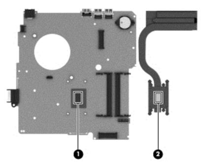
8. Reverse this procedure to install the fan/heat sink assembly. Replace the thermal material that ships with the replacement heat sink.
