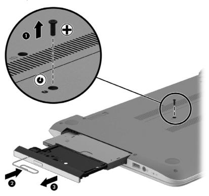
If it is necessary to replace the optical drive bracket and bezel, position the optical drive with the rear panel toward you.
