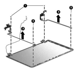
**3.** If it is necessary to replace the display panel cable:
