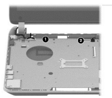
2. Remove the Phillips PM2.5×6.5 screw (1) that secures the power connector bracket to the base enclosure. Remove the power connector bracket (2).
