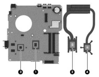
Reverse this procedure to install the heat sink assembly on computer models equipped with switchable discrete graphics.
