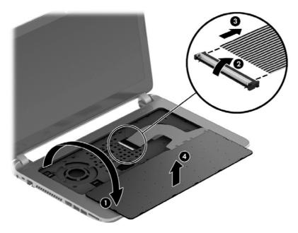
Reverse this procedure to install the keyboard.
