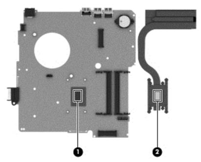
Reverse this procedure to install the heat sink assembly on computer models equipped with UMA graphics.
