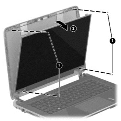
Release the tab (1) and disconnect the display panel cable connector (2). Lift the panel (3) to remove it.
