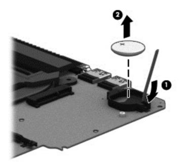
Reverse this procedure to install the RTC battery. When installing the RTC battery, make sure the "+" sign faces up.
