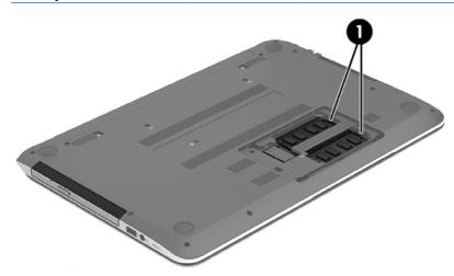
1. Spread the two retaining tabs (1) on each side of the memory module slot to release the memory module. (The memory module tilts up.)
