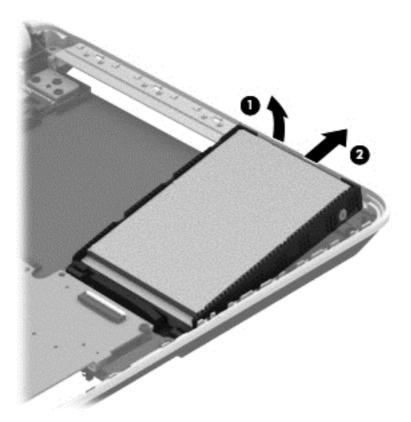
3. Disconnect the hard drive connector cable from the hard drive, and then remove the hard drive.
