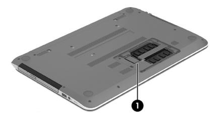
Remove the WLAN module:
