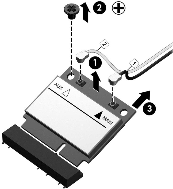
**NOTE:** If the WLAN antennas are not connected to the terminals on the WLAN module, the protective sleeves should be installed on the antenna connectors, as shown in the following illustration.
