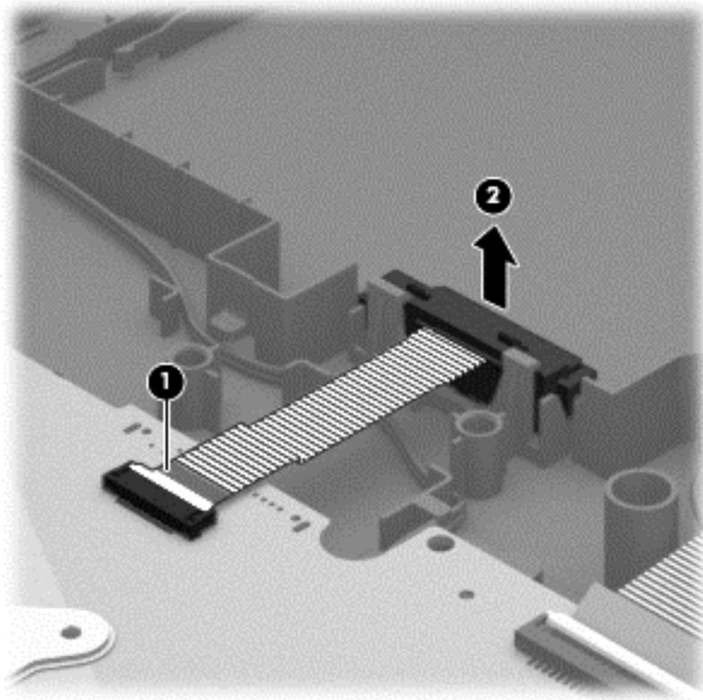
Reverse this procedure to install the optical drive connector cable.
