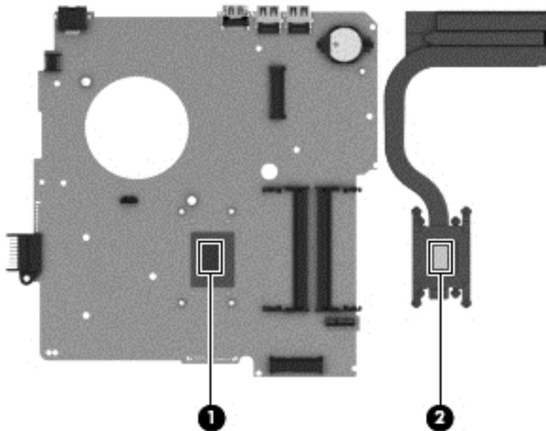
8. Reverse this procedure to install the fan/heat sink assembly. Replace the thermal material that ships with the replacement heat sink.
