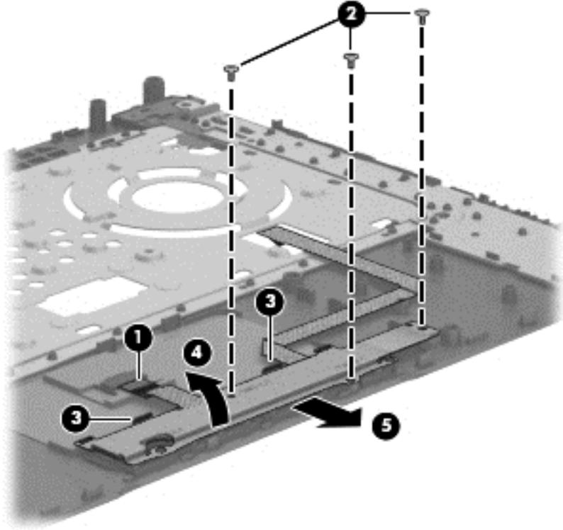
Reverse this procedure to install the TouchPad button board.
