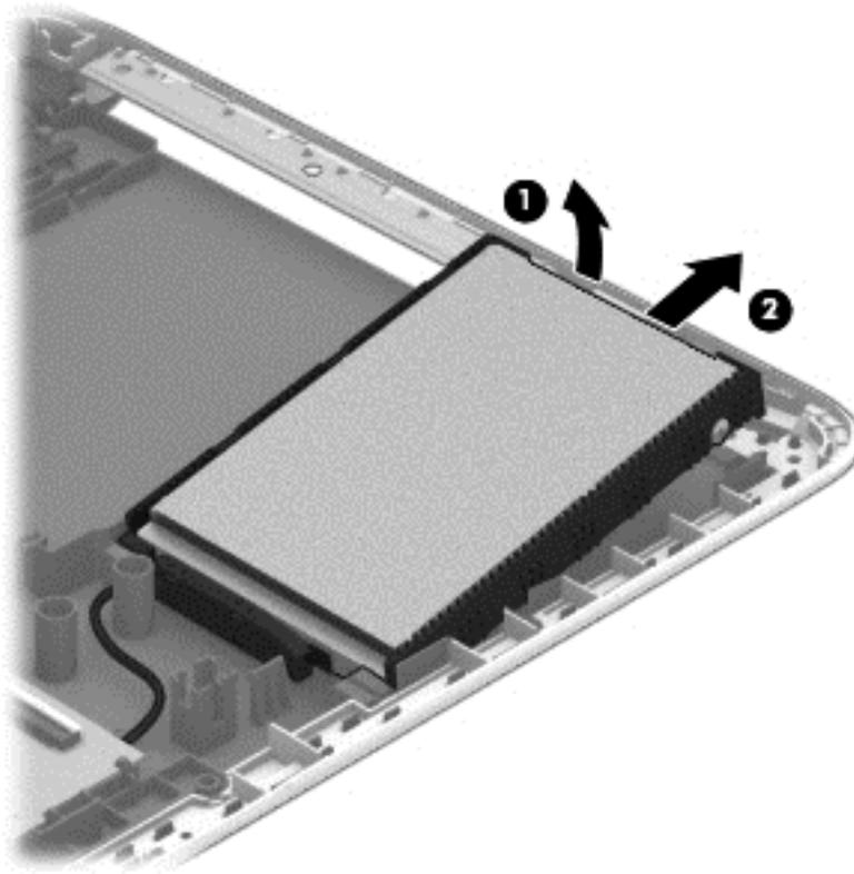
3. Release the hard drive connector cable from the clips.
