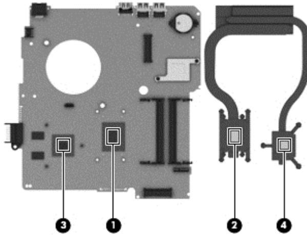
6. Following the 1, 2, 3, 4 sequence stamped into the fan/heat sink assembly, loosen the four Phillips M2.0×10.0 captive screws **(1)** that secure the fan/heat sink assembly to the system board.
