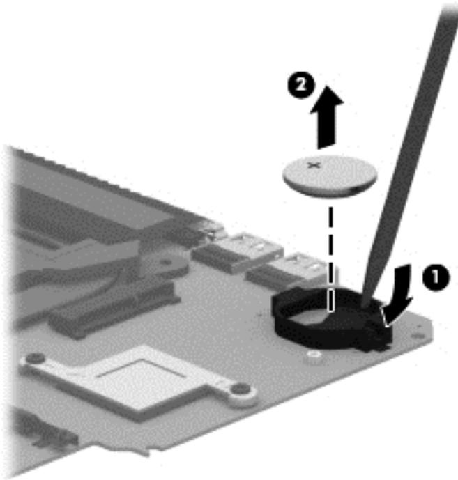
Reverse this procedure to install the RTC battery. When installing the RTC battery, make sure the “+” sign faces up.
