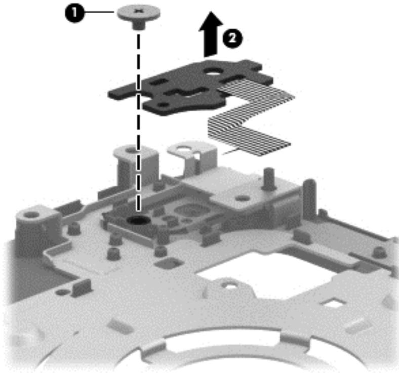
Reverse this procedure to install the power button board.
