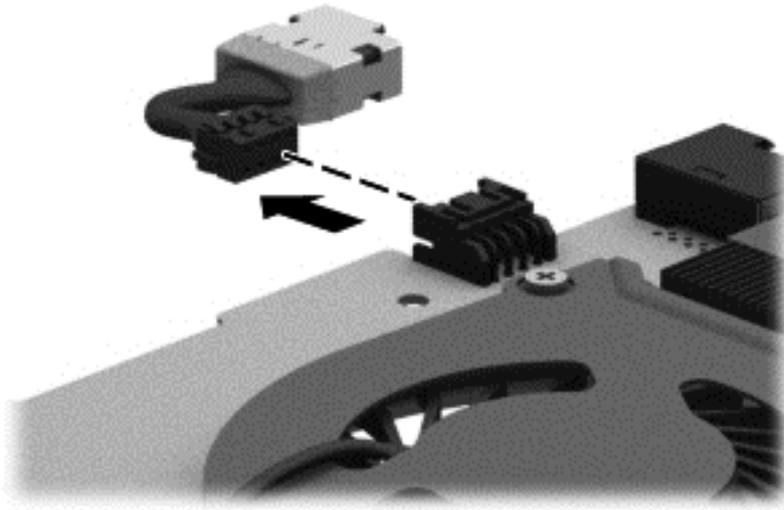
Reverse this procedure to install the power connector cable.
