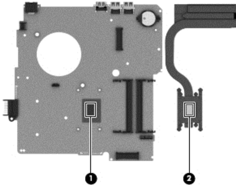
Reverse this procedure to install the heat sink assembly on computer models equipped with UMA graphics.
