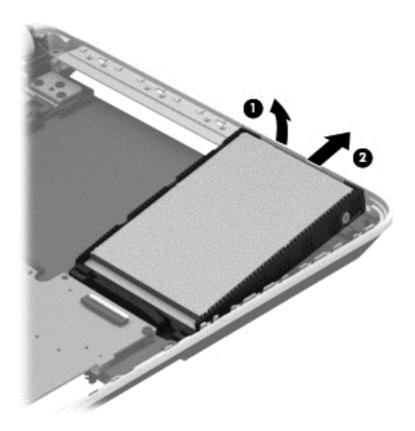
3. Disconnect the hard drive connector cable from the hard drive.
