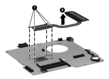
7. Remove the thermal material. The thermal material must be thoroughly cleaned from the surfaces of the heat sink assembly and the system board components each time the heat sink assembly is removed. Replacement thermal material is included with the heat sink assembly and system board spare part kits. Thermal paste is used on the processor (1) and the heat sink assembly section (2) that services it.
