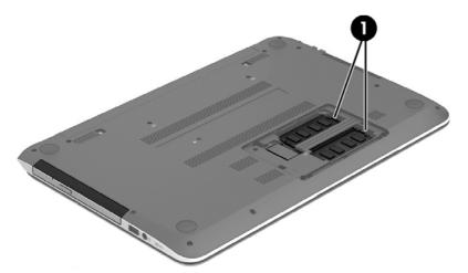
1. Spread the two retaining tabs (1) on each side of the memory module slot to release the memory module. (The memory module tilts up.)
