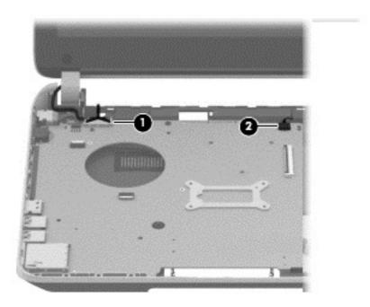
2. Remove the Phillips PM2.5×6.5 screw (1) that secures the power connector bracket to the base enclosure. Remove the power connector bracket (2).
