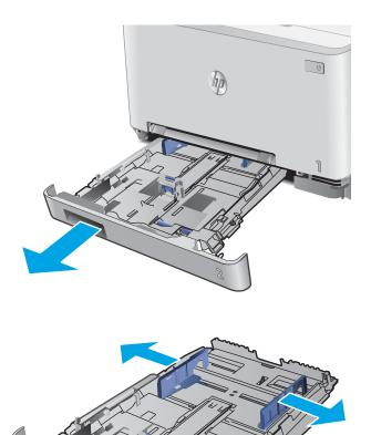
2. Adjust the paper guides by sliding the guides to the size of the paper being used.
