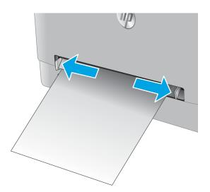
2. Place the right edge of the envelope, face-up, at the opening, and then adjust the side guides so that they lightly touch the envelope, but do not bend it.
