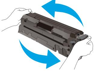
8. Insert the new toner cartridge into the drawer. Make sure that the color chip on the cartridge matches the color chip on the drawer.
