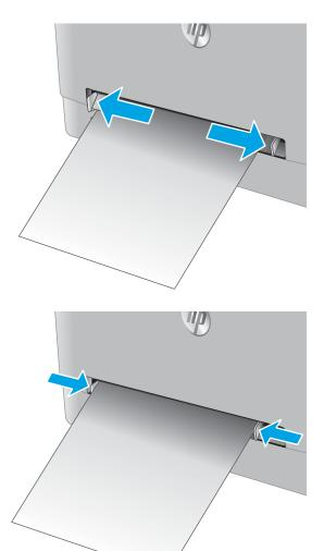
2. Place the top edge of the sheet at the opening, and then adjust the side guides so that they lightly touch the sheet, but do not bend it.
