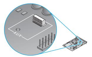
6. Hold the TPM by the edges as shown and align the connector on the TPM with the connector on the formatter. Gently position the TPM on the connector on the formatter. Apply slow, steady, downward pressure. You will hear a click when the connectors are fully engaged.
