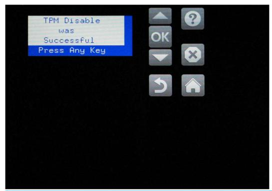
NOTE: Once disabled, the TPM may be left on the formatter or removed. If left installed, it can be reenabled by following the steps in the Install a new or re-enable an existing TPM after disabling a previous TPM section.
