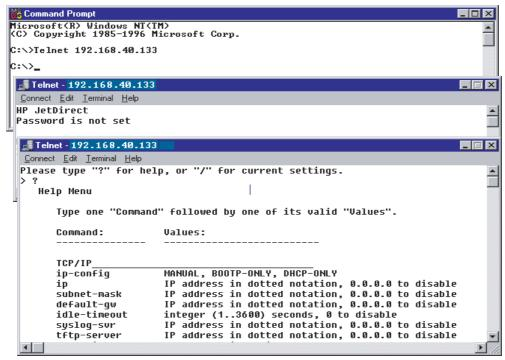
To set configuration parameters, you must set up a Telnet session from your system to the HP Jetdirect print server.
