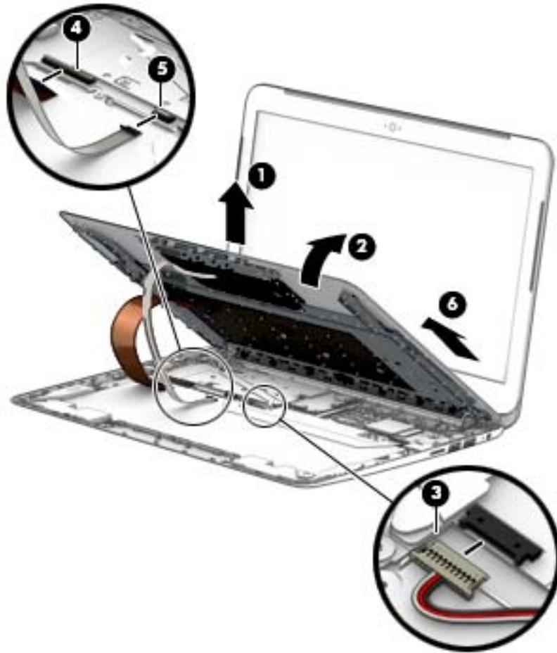
Reverse this procedure to install the keyboard/top cover.
