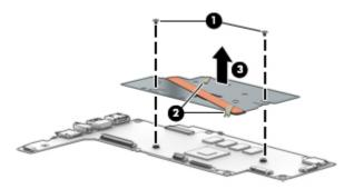
NOTE: The thermal material must be thoroughly cleaned from the surfaces of the system board and the heat sink components each time the heat sink is removed. Thermal paste is used on the processor (1) and the heat sink section (2) that services it.
