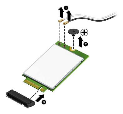
NOTE: If the WWAN antenna is not connected to the terminal on the WWAN module, a protective sleeve must be installed on the antenna connector, as shown in the following illustration.
