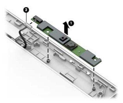
**d.** Remove the webcam/microphone module.
