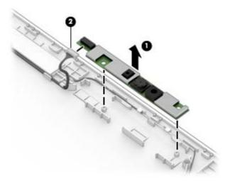
**d.** Remove the webcam/microphone module.
