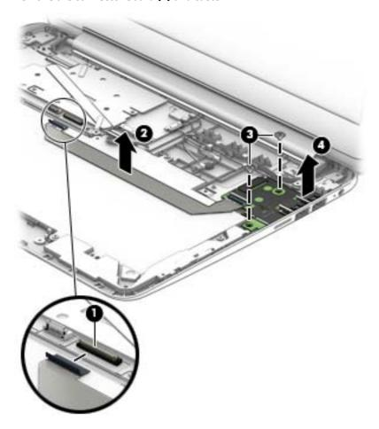
Reverse this procedure to install the connector board.
