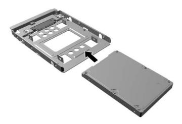
Secure the drive to the bay adapter bracket by installing four black M3 adapter bracket screws through the sides of the bracket into the drive.
