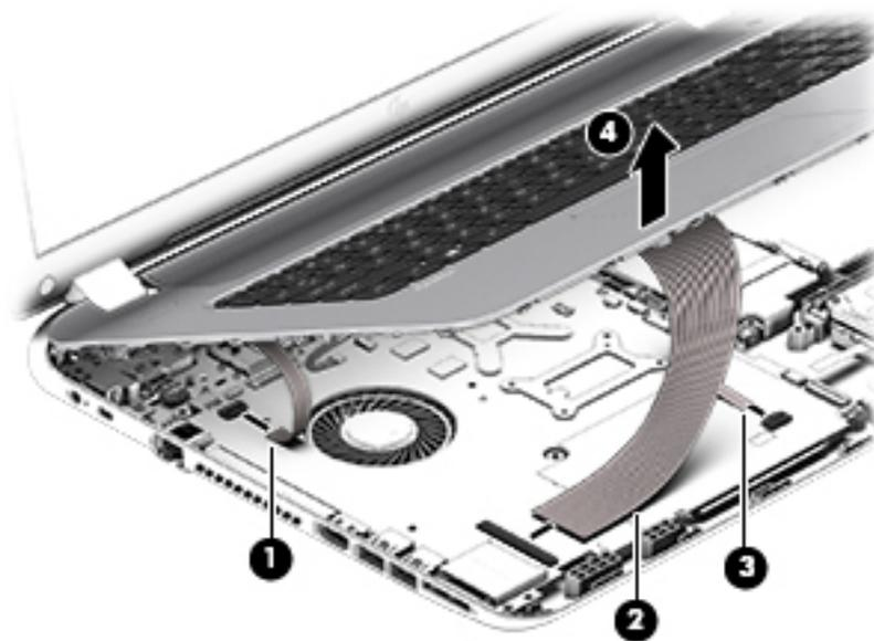
Reverse this procedure to install the top cover and base enclosure.
