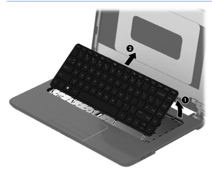
5. Rotate the keyboard over onto the palm rest (1), and the lift the ZIF connector (2) and disconnect the keyboard cable from the system board (3).
