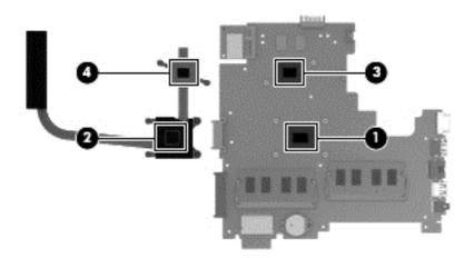
• UMA graphics: Thermal paste is used on the processor (1) and the heat sink (2).
