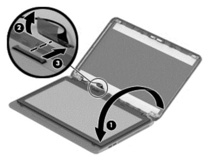
Reverse this procedure to reassemble and install the display bezel, webcam/microphone module, and display panel.
