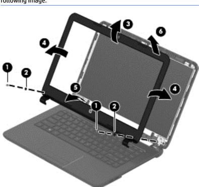
**NOTE:** In this procedure, the display will NOT be connected to the computer, as shown in the following image.
