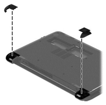
4. Remove the two Phillips broadhead PM2.0×2.0 screws from the optical drive bay that secure the top cover to the computer.
