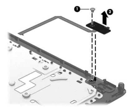
Reverse this procedure to install the power button board and cable.
