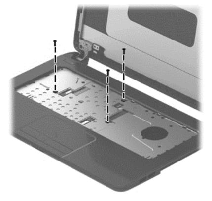
8. Lift the rear edge of the top cover (1) until it disengage from the base enclosure.
