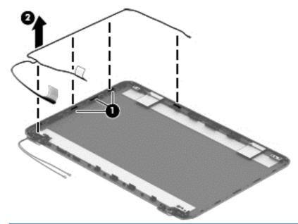
NOTE: If replacing the display enclosure, be sure that the subcomponents (including the webcam/ microphone module, the antenna receivers, and all associated cables and hardware) are transferred to the new enclosure.
