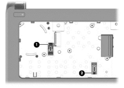
7. Remove the three Phillips PM2.5×4.0 screws that secure the top cover to the computer.
