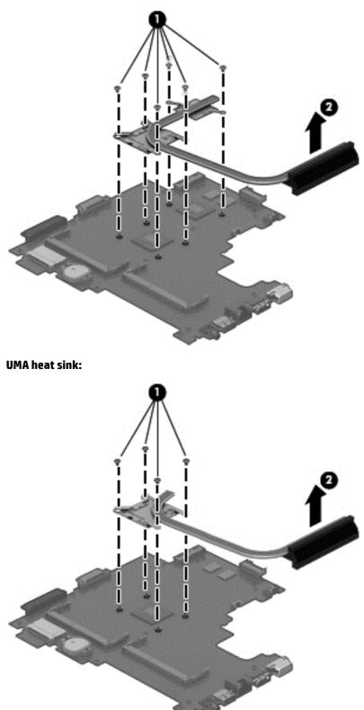
The thermal material must be thoroughly cleaned from the surfaces of the heat sink and the system board components each time the heat sink is removed. Replacement thermal material is included with the heat sink, processor, and system board spare part kits.
