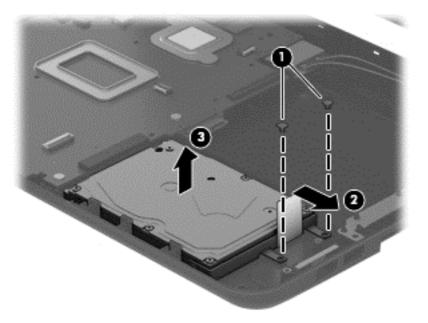
5. To remove the hard drive bracket, remove the two Phillips PM3.0×4.0 screws (1) that secure the bracket to the hard drive.
