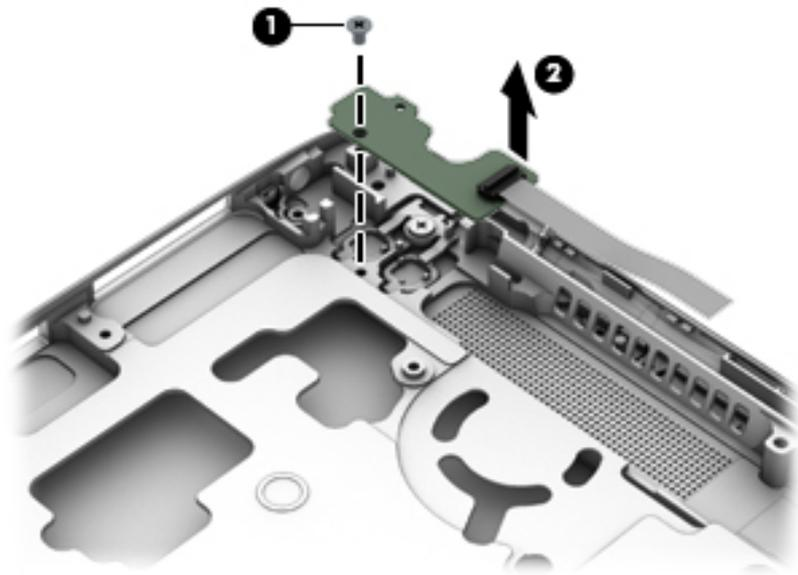
Reverse the removal procedures to install the function board.
