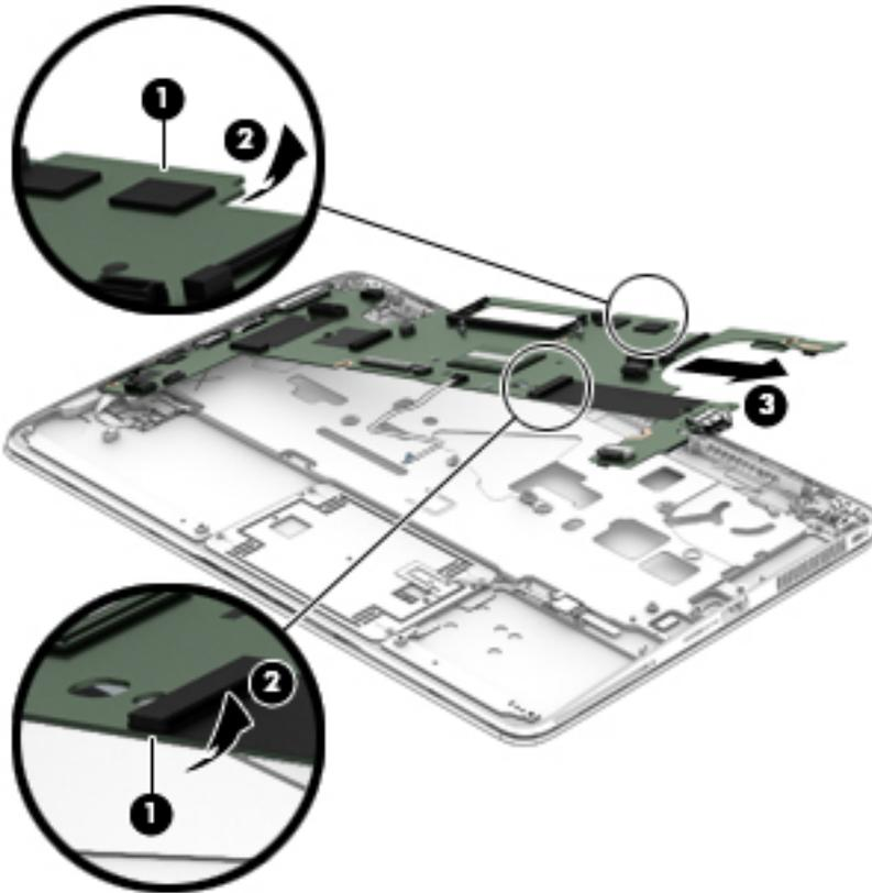
Use the following image to determine all Mylar locations on the system board.
