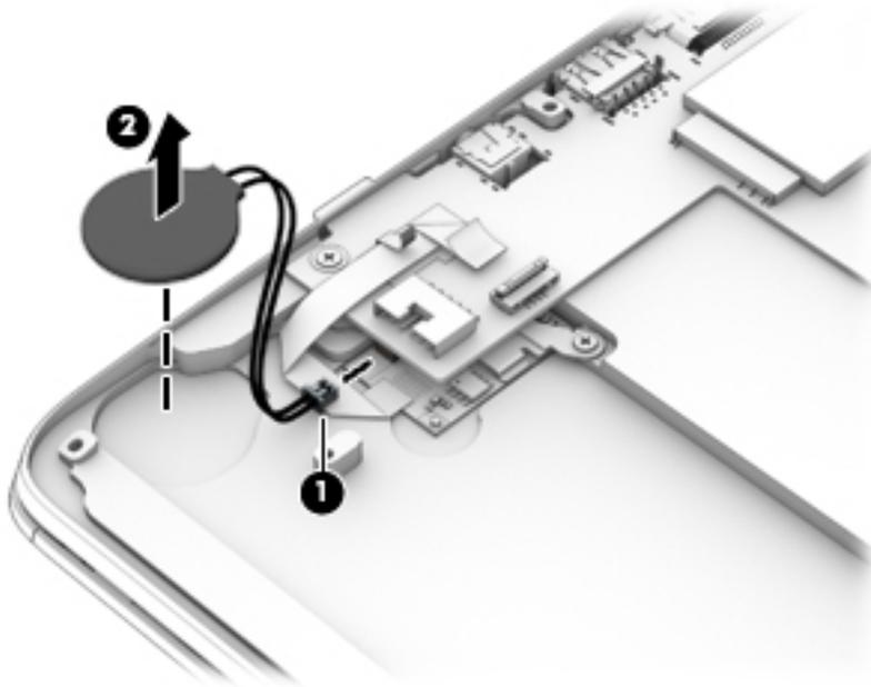
3. Remove the RTC battery.
