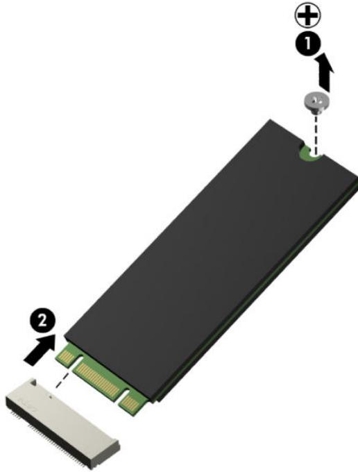
Reverse this procedure to reassemble and install the mSATA drive.
