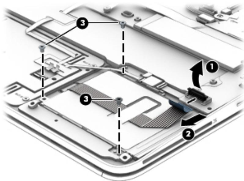
3. Rotate the bottom up the reader upward at an angle **(1)**, and then remove it from the computer **(2)**.
