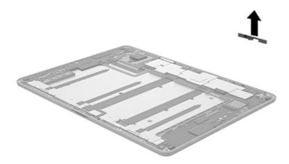
Reverse this procedure to install the volume and power button board.
