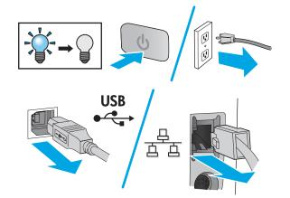
Turn the printer off, and then unplug the power cord and network cables.
