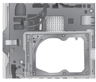
If the optional hard-disk drive (HDD) is installed (as shown above), remove it. If the HDD is not installed, skip this step. If needed, refer to the product support page for your product at <a href="www.hp.com/support">www.hp.com/support</a> for HDD removal instructions.
