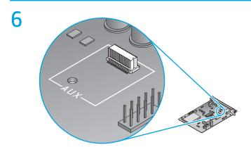
Locate the correct connector on the formatter. The outline of a white square the same size as the TPM is printed on the formatter and surrounds the connector and a hole in the formatter. **NOTE**: The letters **AUX** might not appear on some older boards. The location of the connector on your formatter might be different from the location shown.
