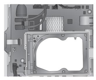
If the optional hard-disk drive (HDD) was not removed, skip this step. If the HDD was removed, reinstall it. If needed, refer to the product support page for your product at www.hp.com/support for HDD installation instructions.
