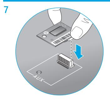
Hold the TPM by the edges as shown and align the connector on the TPM with the connector on the formatter. Gently position the TPM on the connector on the formatter. Apply slow, steady, downward pressure. You will hear a click when the connectors are fully engaged.
