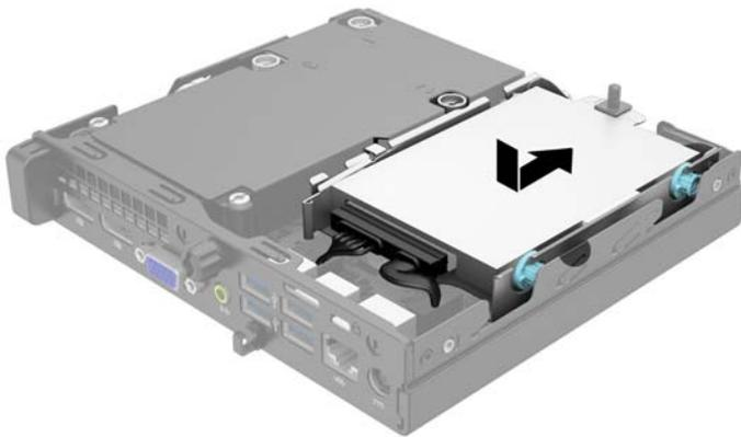
8. Connect the hard drive power cable (1) and data cable (2) to the system board.
