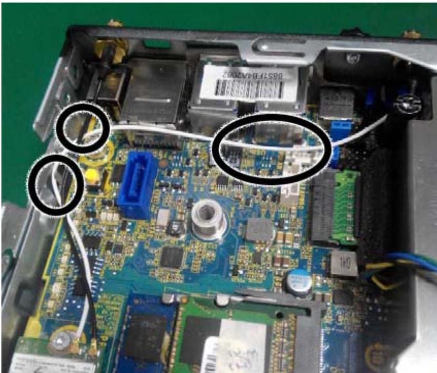
Note the correct cable routing in the following image.
