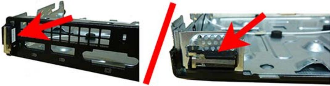
12. Remove the front transceiver from the inside of the computer by pressing the tab to disengage the transceiver and removing the transceiver (arrow in following image points to the tabs on the inside of the computer).
