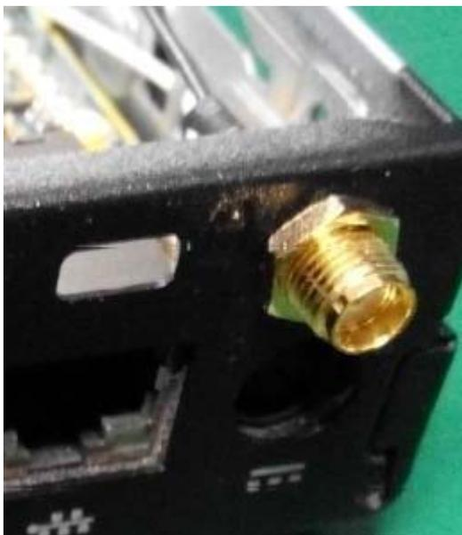
9. Connect the connector on the end of the black antenna cable to the connector labeled '1' on the WLAN module.
