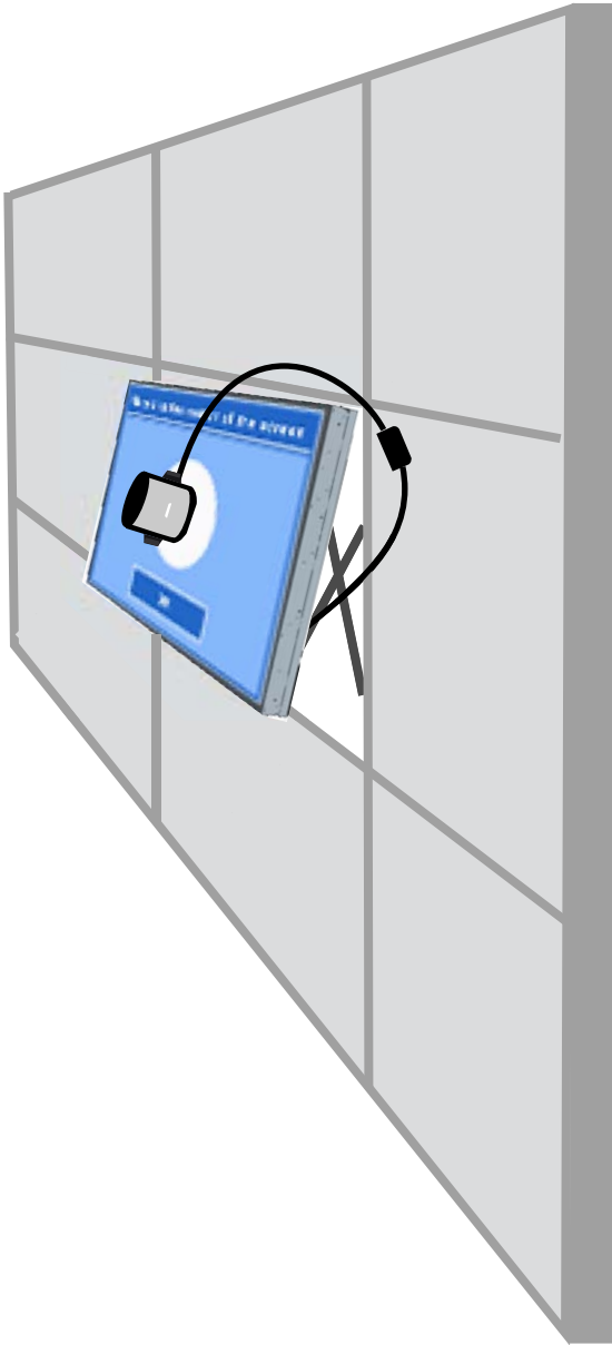
Figure 4-11 Positioning the colorimeter
