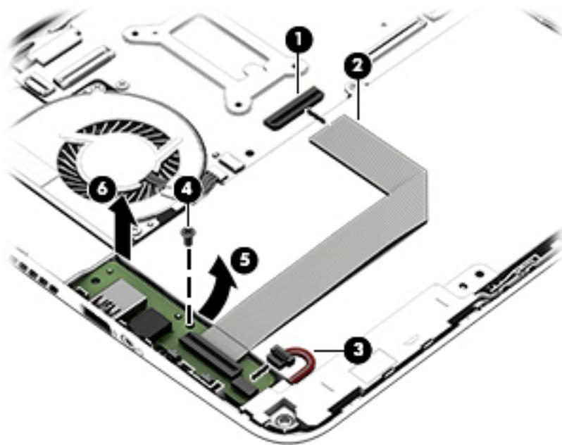
Reverse this procedure to install the audio/USB board.
