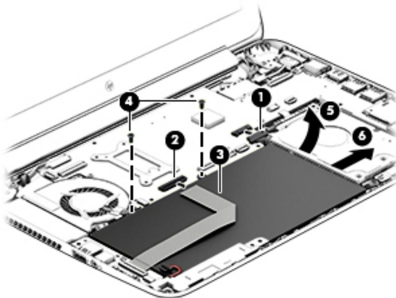
Reverse this procedure to install the battery.
