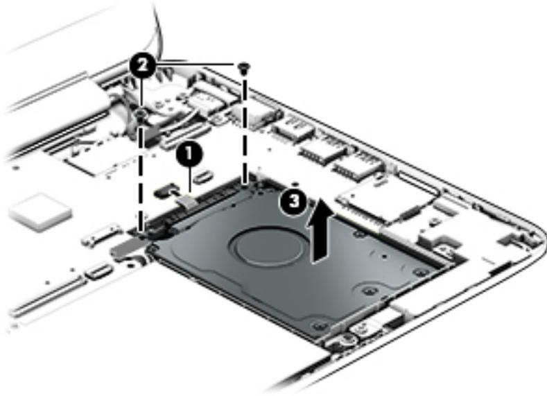
4. If it is necessary to replace the hard drive bracket, release the sides **(1)** of the bracket from the hard drive, and then lift the bracket straight up **(2)** and remove the bracket from the hard drive.
