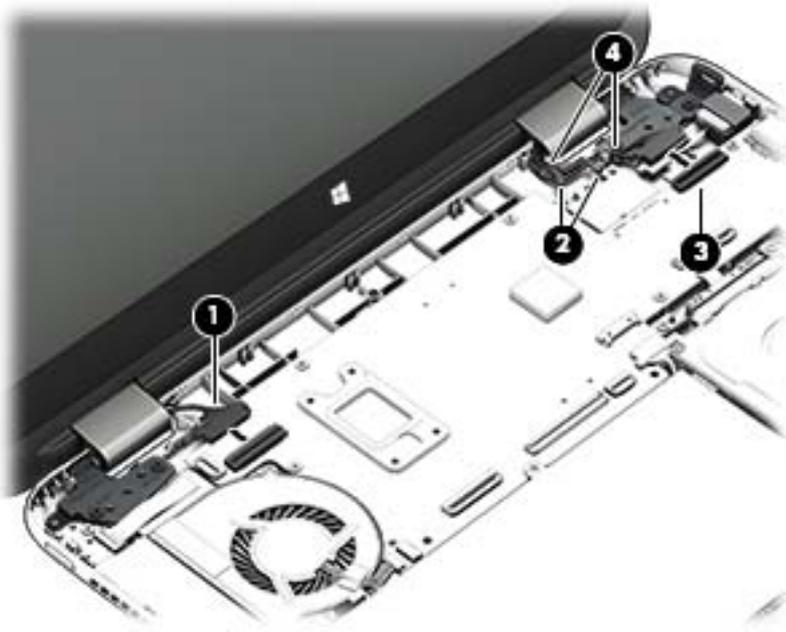
5. Remove the three Phillips PM2.5×5.7 screws **(1)** and the Phillips PM2.5×3.3 screw **(2)** that secure the display assembly to the bottom cover.
