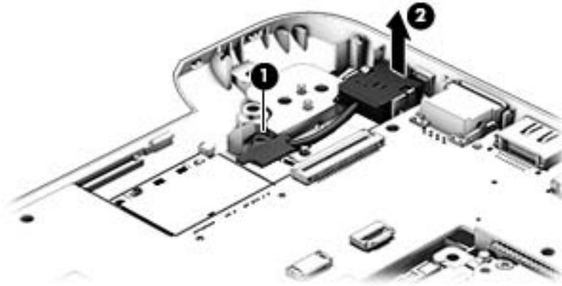
3. Remove the power connector cable.
