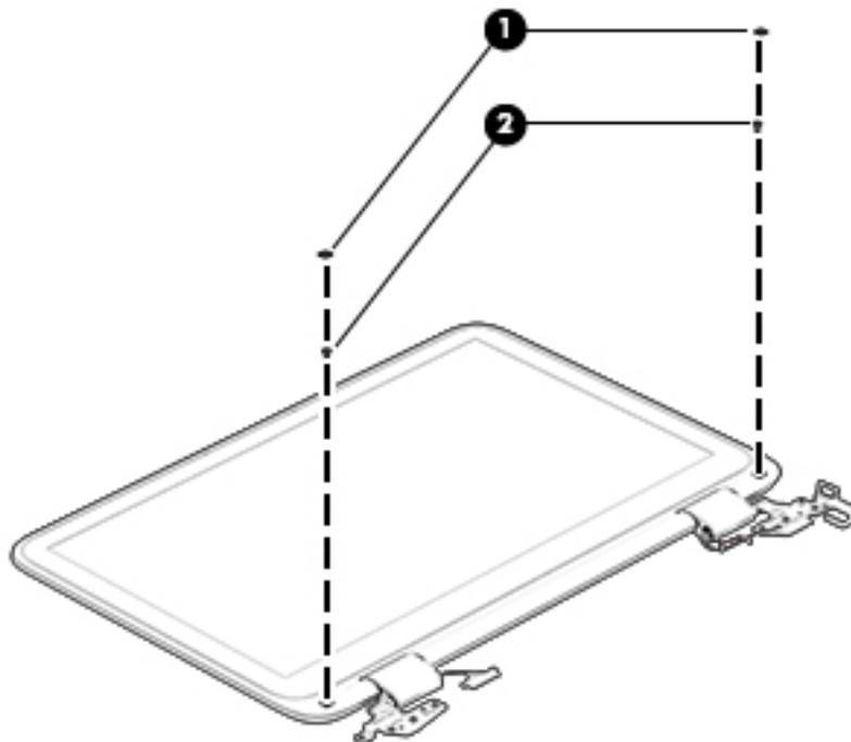
8. Release the top edge of the display panel **(1)** by pulling it away from the back cover.
