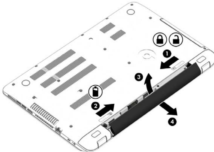
Reverse this procedure to install the battery.
