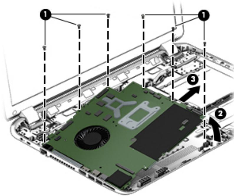
6. Turn the system board over and remove the solid state drive before replacing the system board. Reverse this procedure to install the system board.
