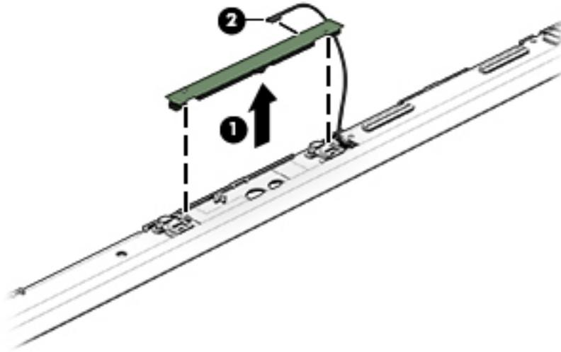
If the computer is equipped with a 3D camera, lift the module **(1)** from the adhesive holding it in place on the display bezel and disconnect the module connector **(2)** from the end of the module if you have not already done so when removing the display cable.
