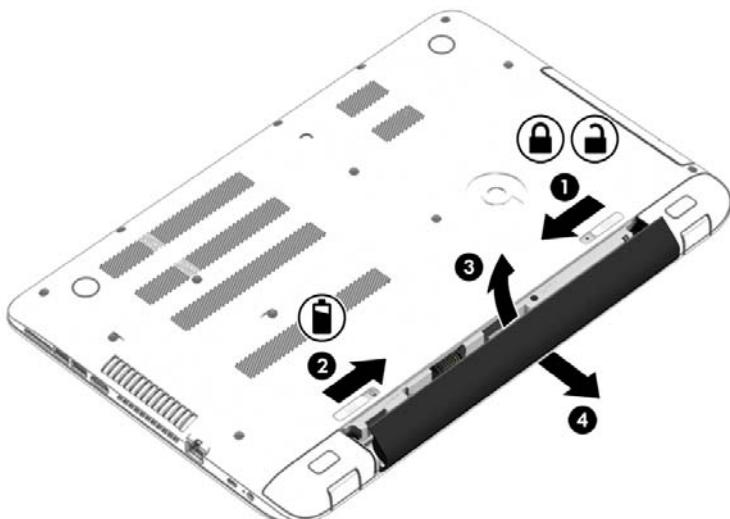
Reverse this procedure to install the battery.
