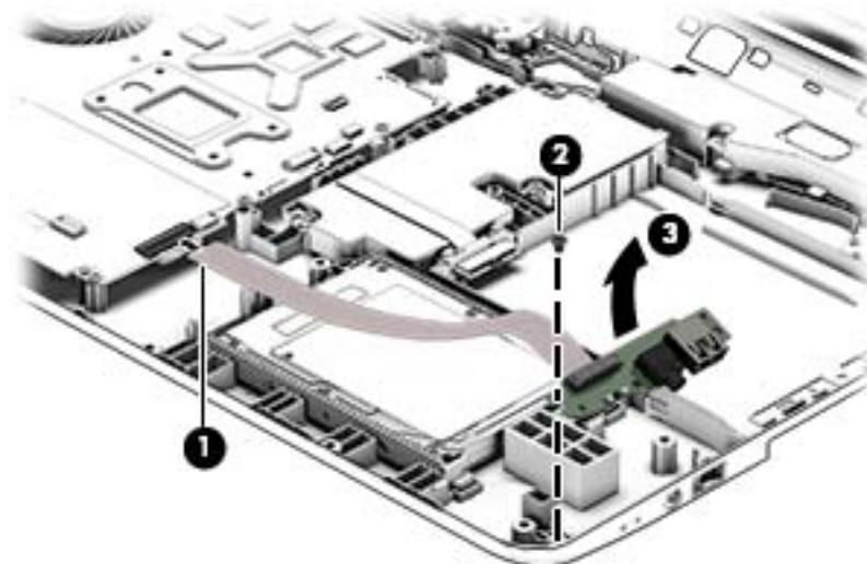
Reverse this procedure to install the USB board and cables.
