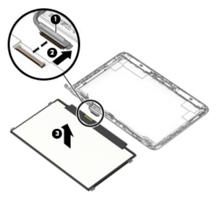
**9.** If it is necessary to replace the display panel cable:
