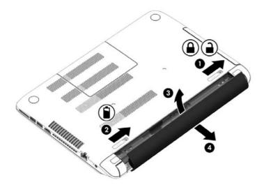
Reverse this procedure to insert the battery.
