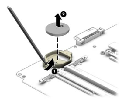
Reverse this procedure to install the RTC battery. When installing the RTC battery, make sure the "+" sign faces up.
