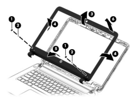
Remove the four Phillips M2.0×2.5 screws (1) and lift the top edge of the display panel (2).
