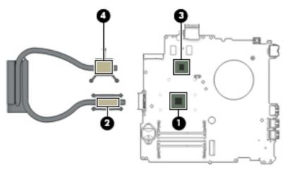
Reverse this procedure to install the heat sink assembly on computer models equipped with switchable discrete graphics.
