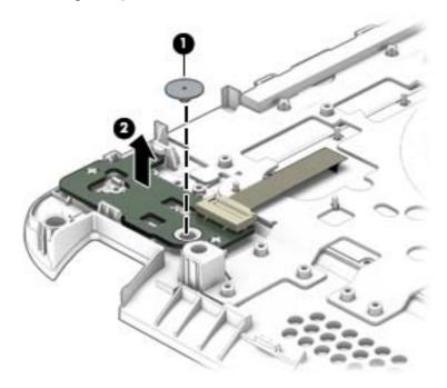
Reverse this procedure to install the power button board.
