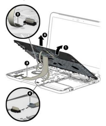
When replacing the top cover, be sure that the following components are removed from the defective top cover and installed on the replacement top cover:
