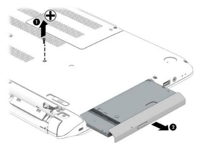
If it is necessary to replace the optical drive bracket and bezel, position the optical drive with the rear panel toward you.
