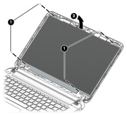
Carefully move the display panel (1) to the keyboard.
