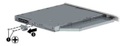
Remove the tab from the drive (1). Rotate the left side of the bezel outward (2), and then remove the bezel (3).
