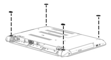
3. Remove the two Phillips M2.5x1.5 screws that secure the rear corner covers (1). Remove the rear corner covers (2). The rear corner covers are included in the Plastics Kit, spare part number 767259-001.
