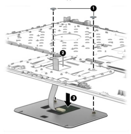
Reverse this procedure to install the TouchPad button board.
