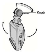
2. Loosen the knob to swivel the camcorder horizontally up to 360°.
