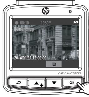
If the Collision Detection function is enabled and a collision is detected, the device will automatically trigger the emergency recording.
