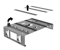
Route the Desktop Mini power cables out the rear of the tray **1** and place the power supply onto the tray **2**.
