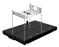
Secure two power supplies at a time by inserting a cable tie (customer provided) through the holes in the brackets on the tray and wrapping the cable tie around the power supplies.
