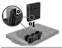
△ CAUTION: You must pull the arm back before inserting the Desktop Mini or the arm may shift the foot on the Desktop Mini out of position. Repeat steps 1 through 6 to install the remaining kit contents and Desktop Minis.
