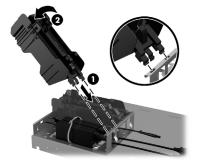
6 Pull back the arm on the rack mount **①** and place the Desktop Mini into the rack mount **②** so that the arm clips into the screw hole on the Desktop Mini.
