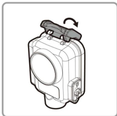
4. Then push the buckle ring on top of the Waterproof Case down and forward so it is in the fixed position.
