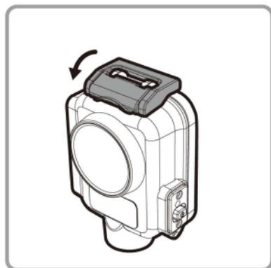
5. Make sure that there is no gap in the Waterproof Case, and that the buckle ring has tightly fixed the Waterproof Case.
