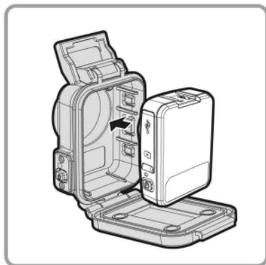
2. Lift up the buckle ring on top of the casing and confirm that the camcorder is firmly installed in the front casing; then close the back cover.
