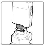
Install the rubber part of the bike mount around the handlebar then pass through the bolt until the mount is firmly fixed.
