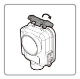
Then push the buckle ring on top of the Waterproof Case down and forward so it is in the fixed position.
