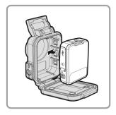
Lift up the buckle ring on top of the casing and confirm that the camcorder is firmly installed in the front casing; then close the back cover.
