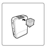
2. Make sure that the tripod adapter is firmly fixed to the camcorder.
