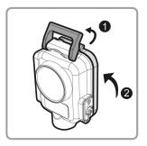
3. Push the buckle on top of Waterproof Case backwards to engage the latch-hook on the back cover.
