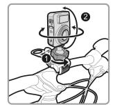
5. Tighten the knob, make sure the device is firmly fixed.
