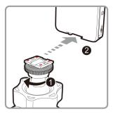
2. Tighten the knob; make sure that the camcorder is firmly fixed.
