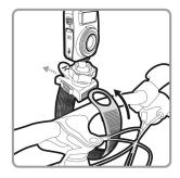
4. Loosen the knob and adjust the camcorder vertically and/or horizontally.
