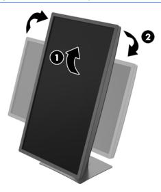
NOTE: To view information on the screen in portrait mode, you can install the HP Display Assistant software included on the software and documentation CD. The position of the OSD menu can also be rotated to portrait mode. To rotate the OSD menu, access the OSD menu by pressing the **Menu** button on the front panel, select **OSD Control** from the menu, and then select **OSD Rotation**.
