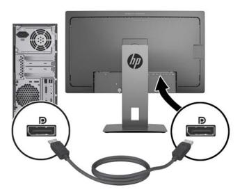
• Connect a Mini-DisplayPort cable to the Mini-DisplayPort connector on the rear of the monitor and the other end to the DisplayPort connector on the source device.
