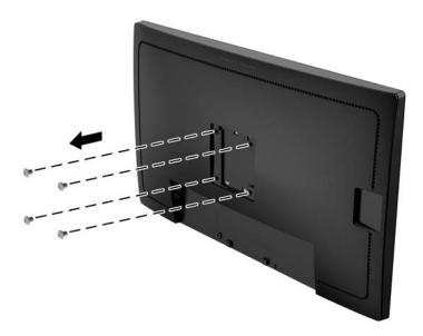
3. Use the four screws removed from the VESA holes on rear of the monitor panel to attach the mounting device to the monitor.
