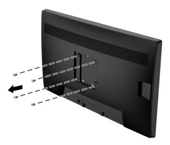
3. Use the four screws removed from the VESA holes on rear of the monitor panel to attach the mounting device to the monitor.
