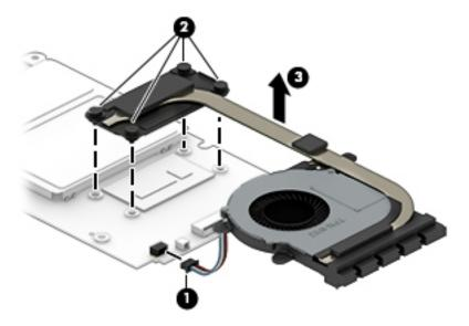
NOTE: The thermal material must be thoroughly cleaned from the surfaces of the fan/heat sink assembly and the system board each time the fan/heat sink assembly is removed. Thermal paste is used on the processor (1) and the fan/heat sink assembly section (2) that services it.
