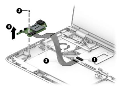
Reverse this procedure to install the connector board.
