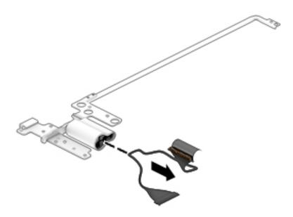
9. If it is necessary to replace the display hinge covers:
