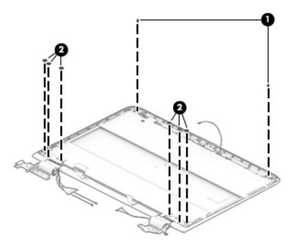
**d.** Rotate the display hinges **(1)** inward until the hinges are clear of the display back cover.
