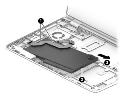
Reverse this procedure to install the battery.
