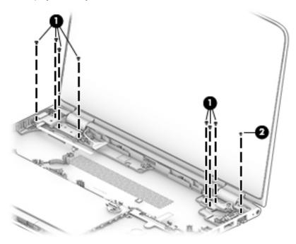
3. Slide the display assembly (1) forward until the display hinges (2) clear the base enclosure.
