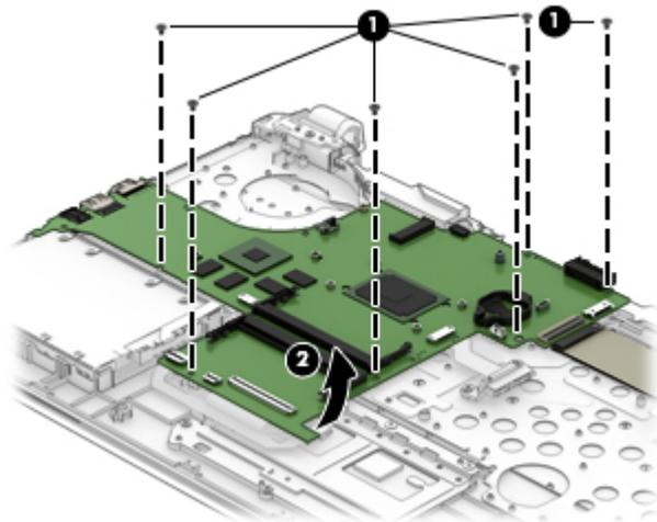
4. Disconnect the USB board cable from the connector under the system board **(1)**, and then remove the system board from the computer **(2)**.
