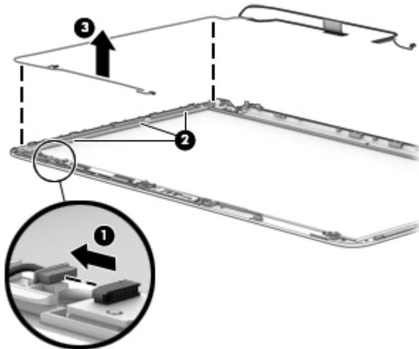
8. If replacing the display enclosure, be sure that the subcomponents (including the webcam/microphone module, the antenna receivers, and all associated cables and hardware) are transferred to the new enclosure.
