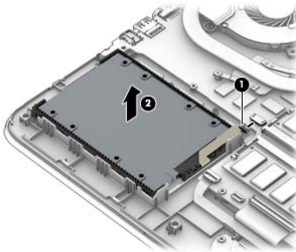
3. To disassemble the hard drive, pull the brackets away from each side of the hard drive **(1)**.
