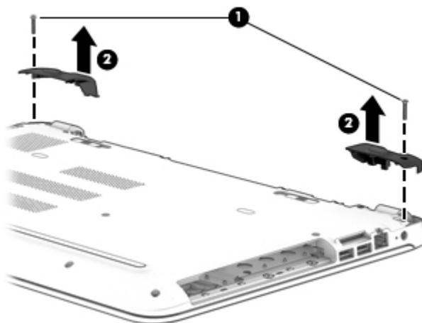
3. Remove the two Phillips PM2.0×2.0 screws from the optical drive bay **(1)**.
