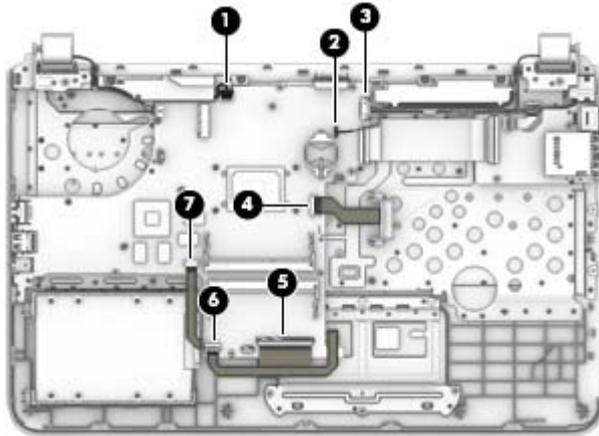
2. Remove the six Phillips PM2.0×3.0 screws (1) that secure the system board to the computer.
