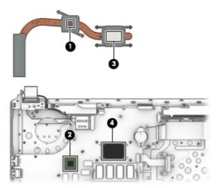
**UMA graphics:** Thermal paste is used on the heat sink (1) and the processor (2).
