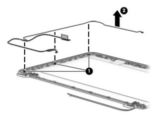
If replacing the display enclosure, be sure that the subcomponents (including the webcam/microphone
