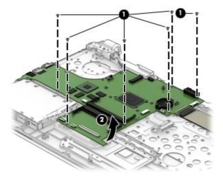
4. Disconnect the USB board cable from the connector under the system board (1), and the remove the system board from the computer (2).
