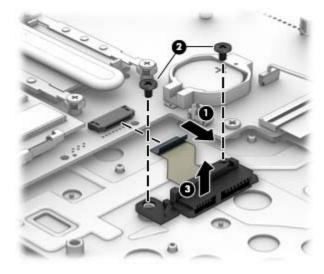
Reverse this procedure to install the optical drive connector.
