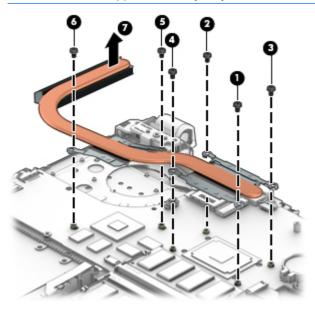
If you have a model with UMA graphics, In the order indicated, remove the four Phillips PM2.0×3.0 screws (1) – (4) that secure the heat sink to the system board. Remove the heat sink (5) from the system board.
