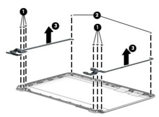
5. To remove the wireless antenna cables and transceivers, release the wireless antenna cables from the clips (1) built into the display enclosure, peel the transceivers from the enclosure (2), and then remove the antenna cables and transceivers (3).
