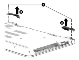
3. Remove the two Phillips PM2.0×2.0 screws from the optical drive bay (1).
