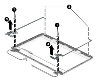
5. To remove the wireless antenna cables and transceivers, release the wireless antenna cables from the clips (1) built into the display enclosure, peel the transceivers from the enclosure, and then remove the antenna cables and transceivers (2).
