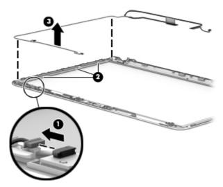
**8.** If replacing the display enclosure, be sure that the subcomponents (including the webcam/microphone module, the antenna receivers, and all associated cables and hardware) are transferred to the new enclosure.
