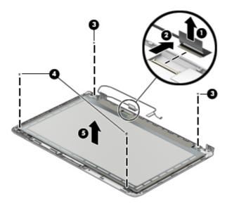
e. Rotate the display panel until it is upside-down next to the display enclosure (1).
