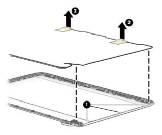
**6.** To remove the display/webcam cable, remove the cable from the clips built into the display enclosure **(1)**, and then remove the cable from the display enclosure **(2)**.
