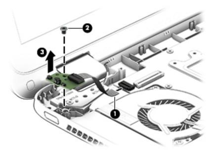
Reverse this procedure to install the power button board and cable.
