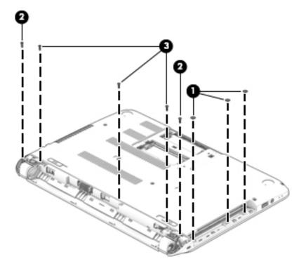
5. Remove the 11 Phillips PM2.5×6.0 screws that secure the bottom cover to the computer.
