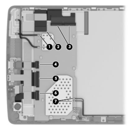
8. Remove the four Phillips PM2.5×3.5 screws (1) that secure the system board to the computer.
