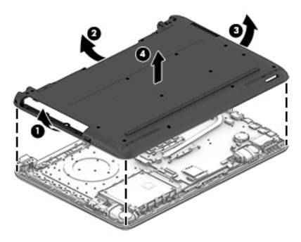
Reverse this procedure to install the bottom cover.
