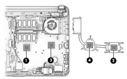
• UMA graphics (Intel Core processors): Thermal paste is used on the heat sink (1) and the processor (2).
