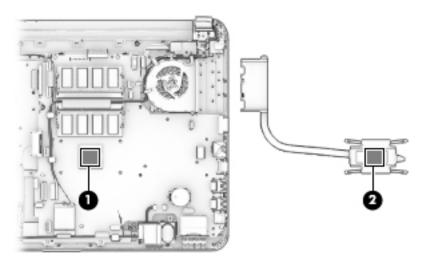
• Intel Pentium and Celeron processors: Thermal paste is used on the heat sink (1) and processor (2).
