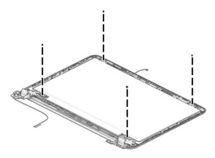
**b.** Rotate the display panel off the display enclosure **(1)** to gain access to the display cable connection on the back of the panel.
