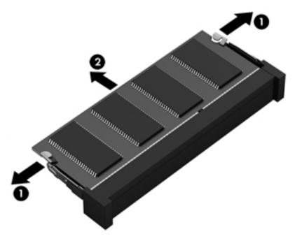
Reverse this procedure to install a memory module.
