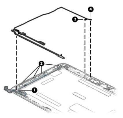
7. If you need to remove the touch control board, disconnect the cables (1)(2) from the board.
