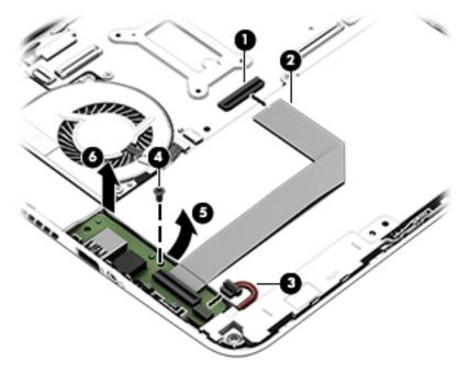
Reverse this procedure to install the USB board.
