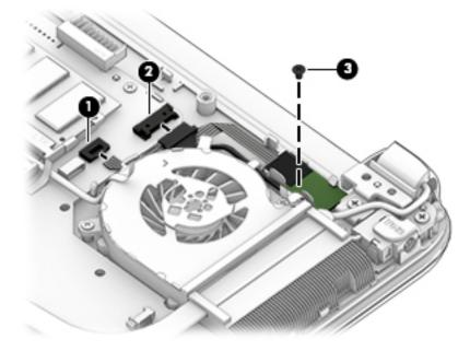
4. Press the tab that secures the board to the computer (1), and then remove the power button board and cable from the computer (2).
