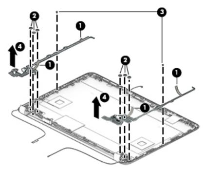
5. To remove the wireless antenna cables and transceivers, release the wireless antenna cables from the clips built into the display enclosure (1), and then remove the cables (2).
