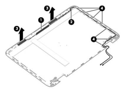
6. To remove the display/webcam cable, remove the cable from the clips built into the display enclosure (1), and then remove the cable from the display enclosure (2).
