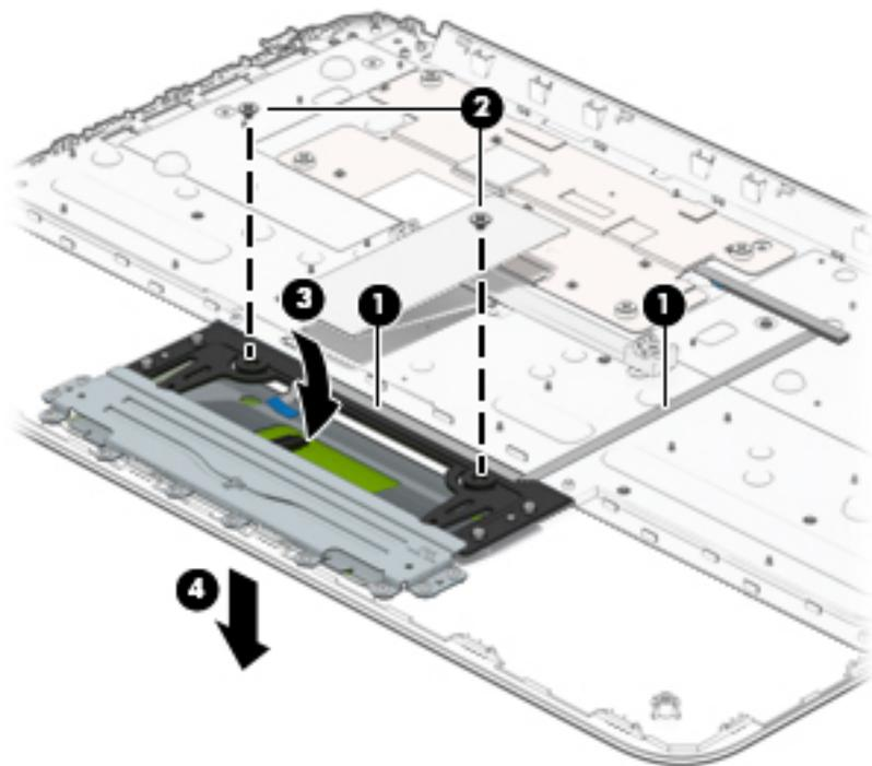
Reverse this procedure to install the TouchPad button board and cables.
