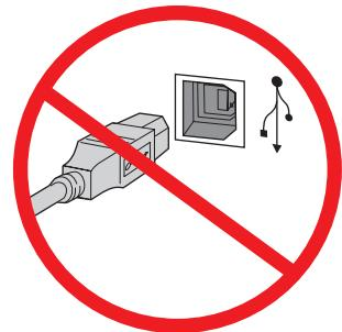
**EN** **Windows:** Do not connect the USB cable until prompted during the software installation in the next step. If the network cable was connected in Step 7, proceed to Step 11.
