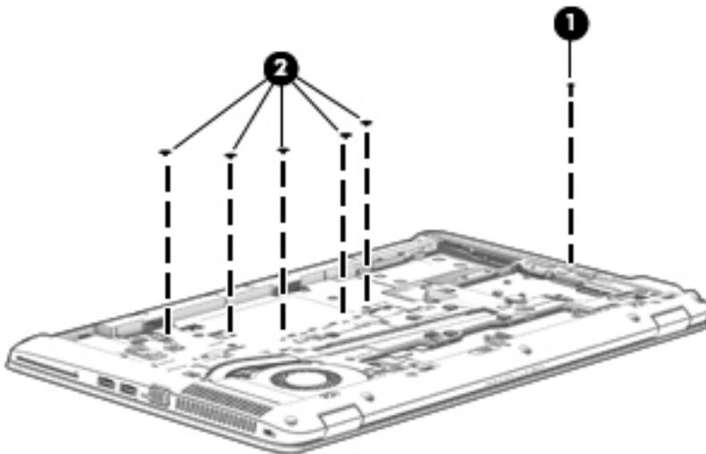
5. Lift the base enclosure off the computer.
