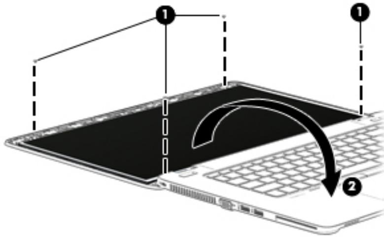
10. Lift the tape that secures the display cable to the display panel **(1)**, and the disconnect the display cable from the panel **(2)**.
