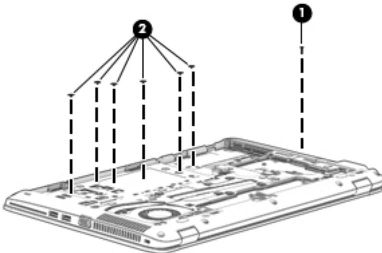
5. Lift the base enclosure off the computer.
