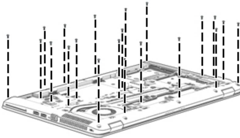
4. Remove the Phillips PM2.0×8.0 screw (1) near the media card reader and the five Phillips PM2.0×5.0 broadhead screws (2) inside the battery bay that secure the base enclosure to the computer.
