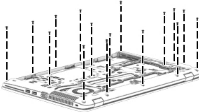
4. Remove the Phillips PM2.0×8.0 screw **(1)** near the media card reader and the six Phillips PM2.0×5.0 broadhead screws **(2)** inside the battery bay that secure the base enclosure to the computer.
