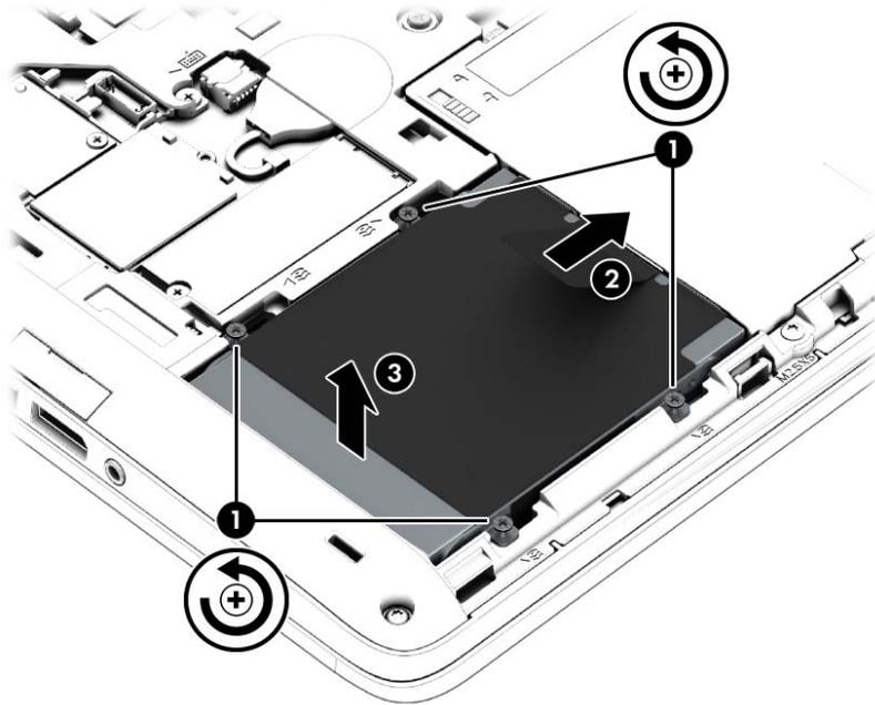
3. If it is necessary to disassemble the hard drive, perform the following steps:
