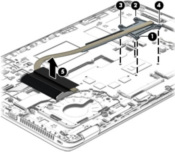
3. The following illustrations show the replacement thermal material locations. The thermal material must be thoroughly cleaned from the surfaces of the heat sink and the system board components each time the heat sink is removed. Replacement thermal material is included with the heat sink, processor, and system board spare part kits.
