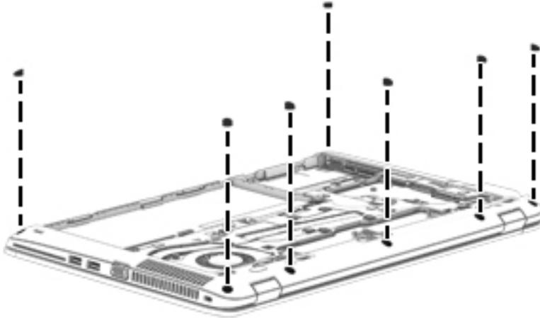
3. Remove the 16 Torx T8M2.5×5.0 screws that secure the base enclosure to the computer.
