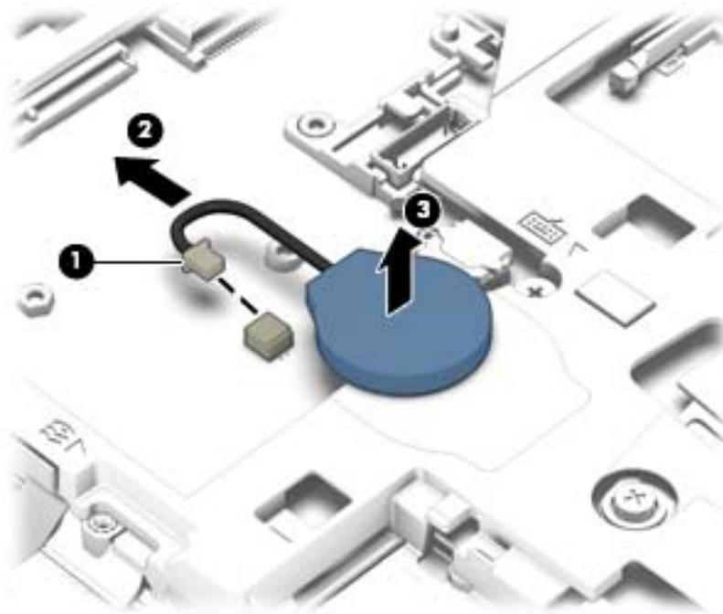
3. Remove the RTC battery.
