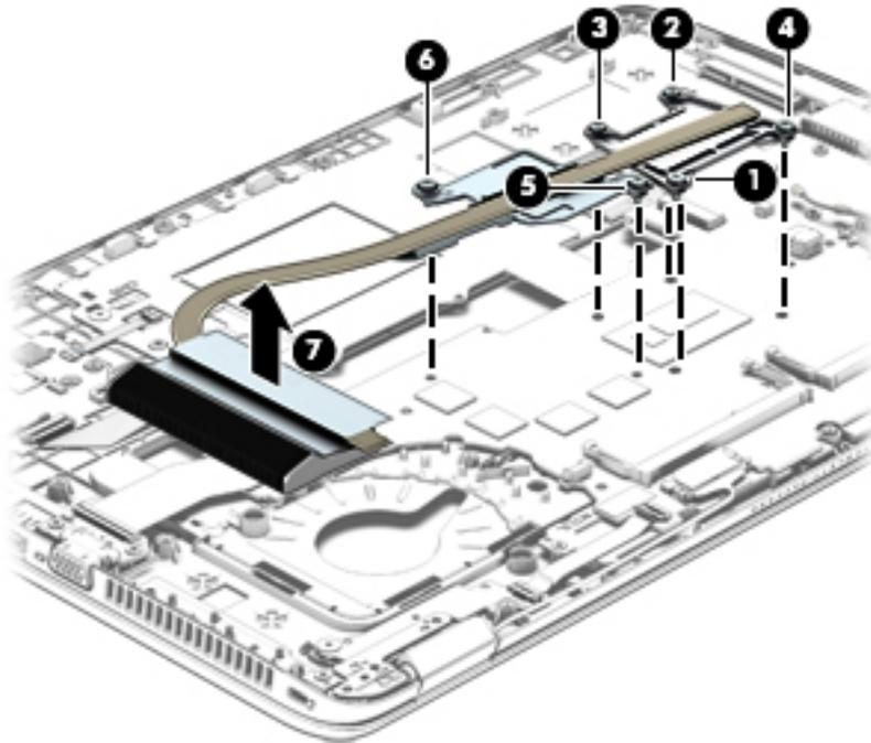
2. Following the 1, 2, 3, 4 sequence stamped into the heat sink, loosen the four captive Phillips screws (1) – (4) that secure the heat sink to the system board, and then remove the heat sink (5).
