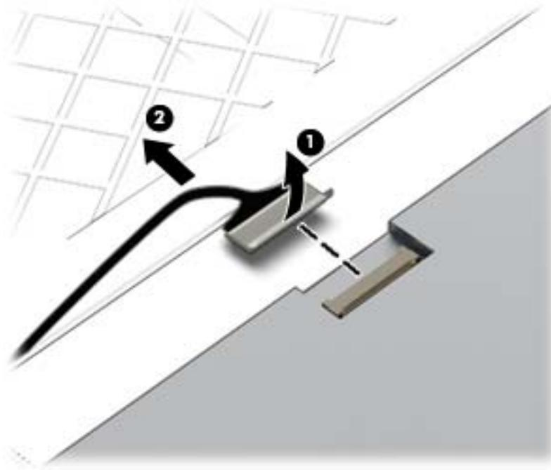
6. Lift the display panel from the display enclosure.
