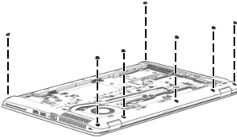
3. Remove the 21 Torx T8M2.5×5.0 screws that secure the base enclosure to the computer.
