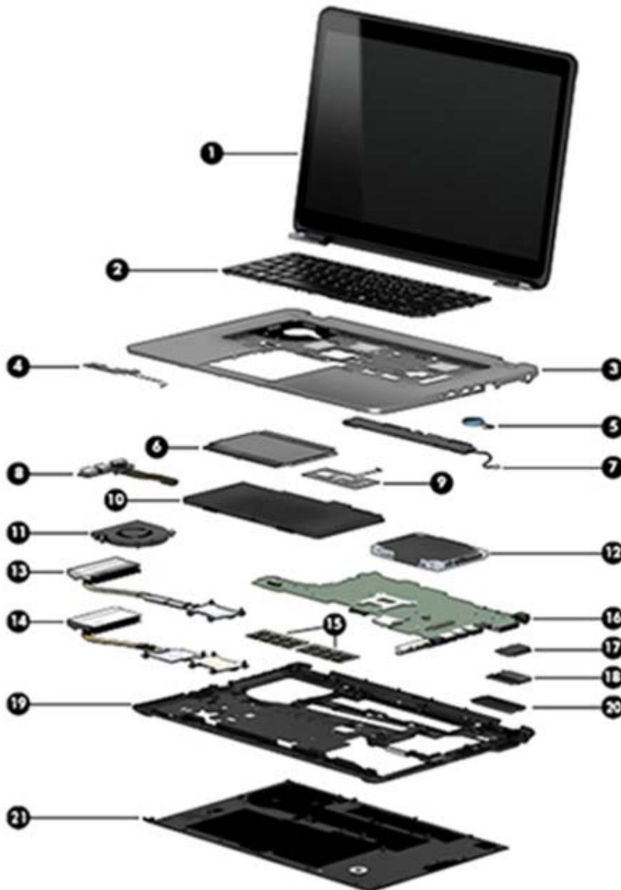
**IMPORTANT:** For system board (16) replacement on serial numbers xxx501xxxx and below, you must use a conversion kit (see product description for “(Gold Conversion Kit)” in the section marked 16a of the table below). For serial numbers xxx502xxxx and above, use the standard spare kit (see product description for “(Gold)”).
