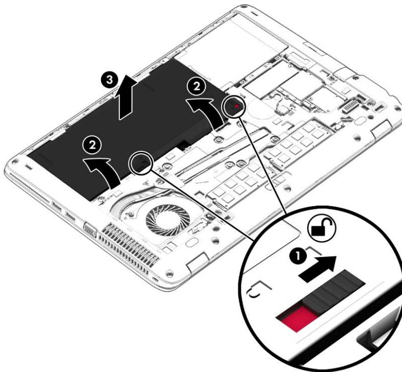
Install the battery by inserting it into the battery bay until you hear a click.
