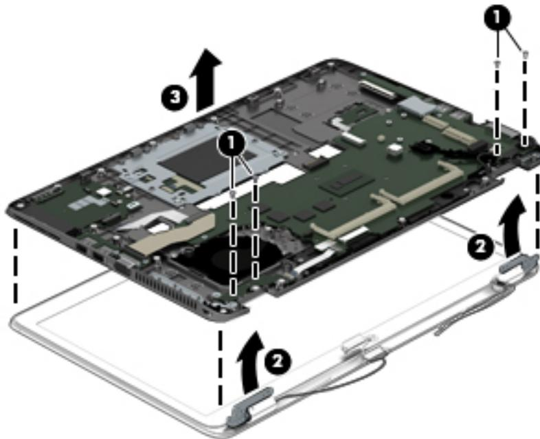
6. If you need to remove the bezel, lift to disengage the bezel on the bottom **(1)**, left and right sides **(2)**, and top **(3)**.
