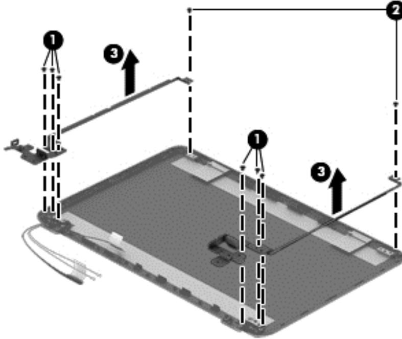
5. To remove the wireless antenna cables and transceivers, release the wireless antenna cables from the clips built into the display enclosure.
