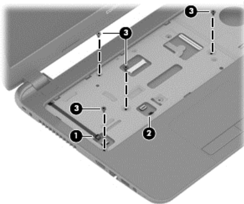
8. Lift the rear edge of the top cover (1) until it disengage from the base enclosure.
