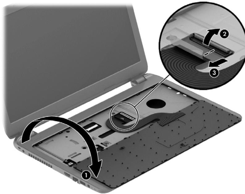
Reverse this procedure to install the keyboard.
