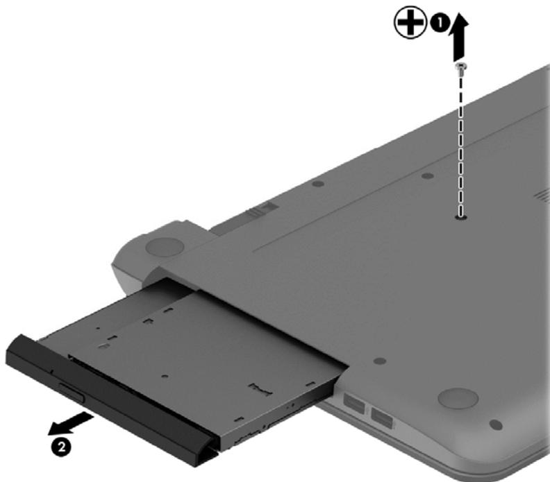
3. If it is necessary to replace the optical drive bracket on the rear of the optical drive, position the optical drive with the rear panel toward you.
