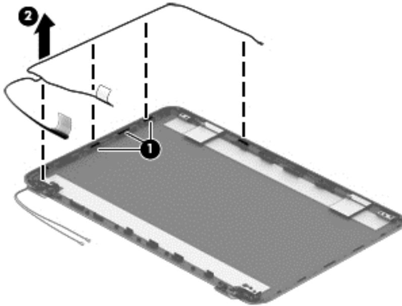
7. If replacing the display enclosure, be sure that the subcomponents (including the webcam/microphone module, the antenna receivers, and all associated cables and hardware) are transferred to the new enclosure.
