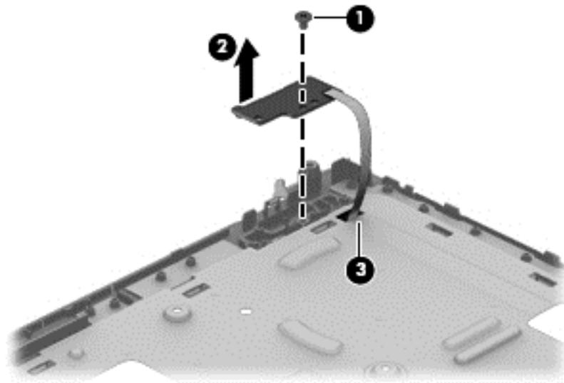
Reverse this procedure to install the power button board and cable.
