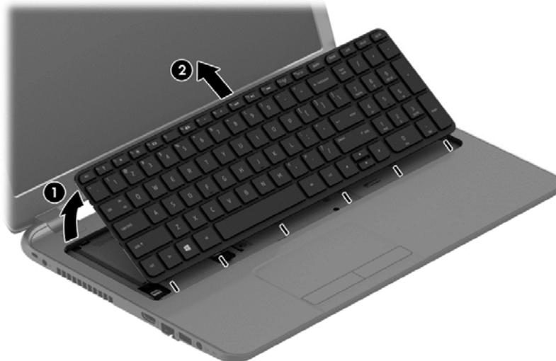
5. Rotate the keyboard over onto the palm rest **(1)**, and the lift the ZIF connector **(2)** and disconnect the keyboard cable from the system board **(3)**.
