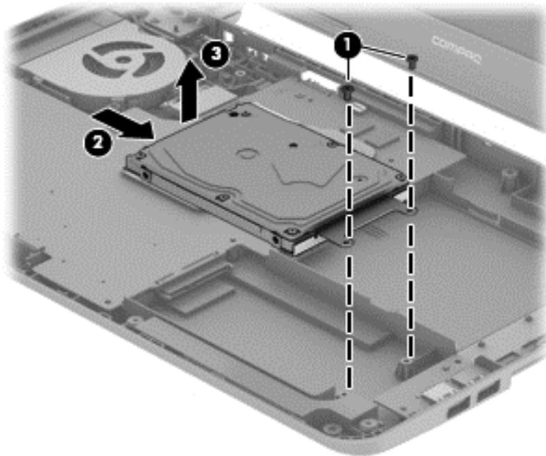
4. To remove the hard drive bracket, remove the two Phillips PM3.0×4.0 screws (1) that secure the bracket to the hard drive.
