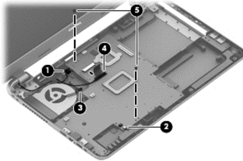
3. Lift the right side of the system board **(1)**, and then pull the board away from the computer enough to disengage the connectors from the side of the base enclosure **(2)**.
