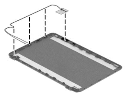
To remove the display/webcam cable, remove the cable from the clips built into the display enclosure (1), and then remove the cable from the display enclosure (2).
