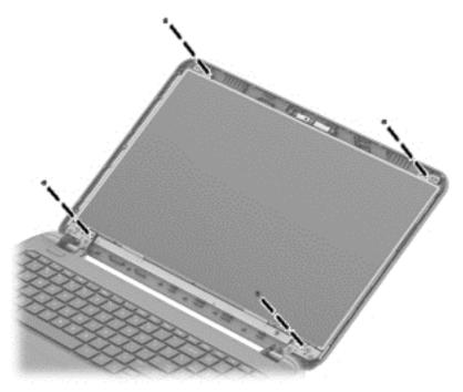
Rotate the display panel onto the keyboard to gain access to the display cable connection on the back of the panel (1).
