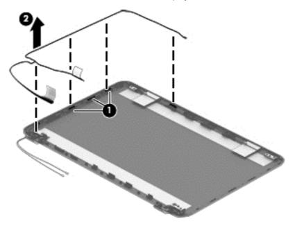
If replacing the display enclosure, be sure that the subcomponents (including the webcam/microphone module, the antenna receivers, and all associated cables and hardware) are transferred to the new enclosure.
