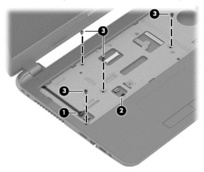
**8.** Lift the rear edge of the top cover **(1)** until it disengage from the base enclosure.
