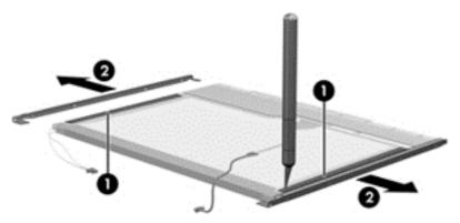
11. Remove the screws (1) that secure the backlight cover to the display panel.
