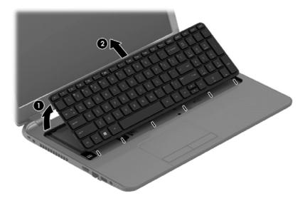
Rotate the keyboard over onto the palm rest (1), and the lift the ZIF connector (2) and disconnect the keyboard cable from the system board (3).
