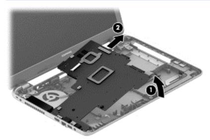
4. Flip the system board upside down to gain access to the speaker connector (1).
