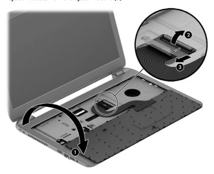
Reverse this procedure to install the keyboard.
