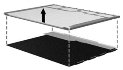
**24.** Recycle the LCD panel and backlight.
