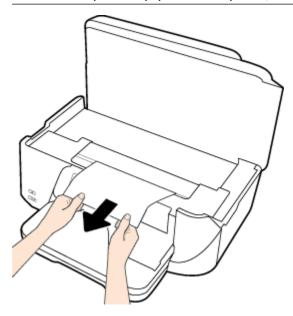
**d.** Move the carriage to the far left of the printer, and do the same as in the previous step to remove any torn pieces of paper.
