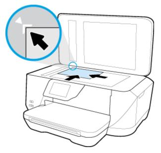
**f.** Follow the instructions on the printer display to align the cartridges. Recycle or discard the cartridge alignment sheet.
