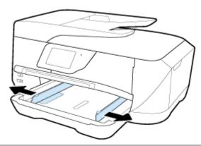
**NOTE:** If the paper is too long, pull out the input tray to extend it to the desired paper size.
