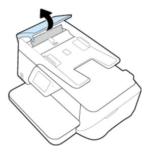
**2.** Lift the blue arrow label located on the front edge of the document feeder.
