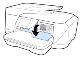
Press the front of the ink cartridge to release it, and then remove it from the slot.
