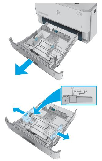
2. Adjust the paper-width guides by squeezing the adjustment latch on the left guide and sliding the guides to the size of the paper being used.
