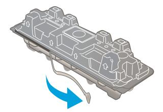
5. Remove the toner cartridge from the opened packaging shell. Place the used toner cartridge in the shell for recycling.
